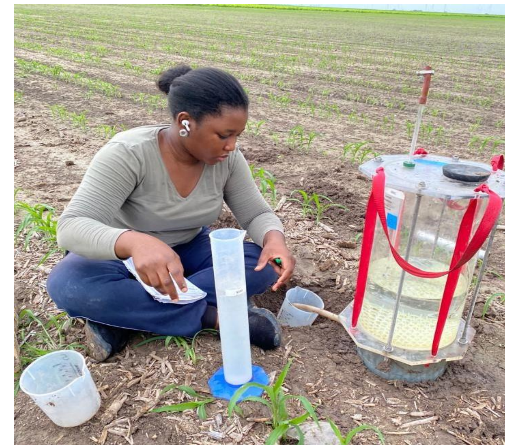
Cornell Infiltrometer test
