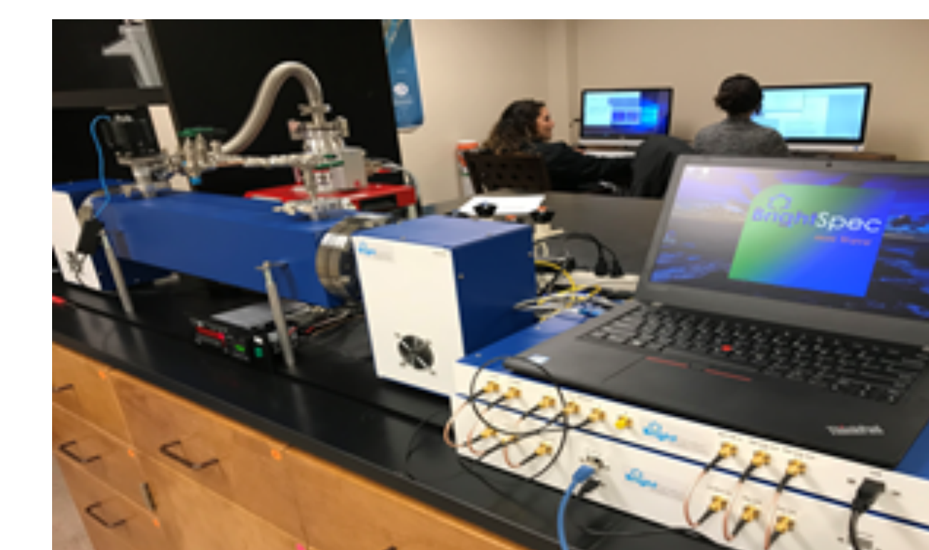
Figure 4. BrightSpec chirped-pulse microwave spectroscopy at UTRGV (18-26 GHz)
