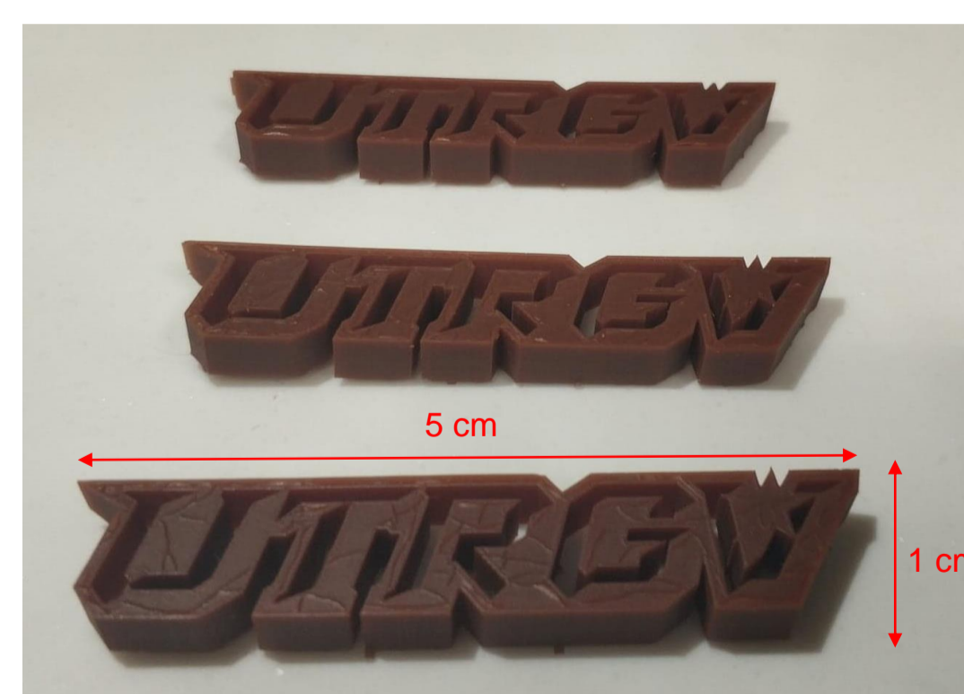
Model printed from Clear resin + barium ferrite nanoparticles (concentration 5 mg/ml)
