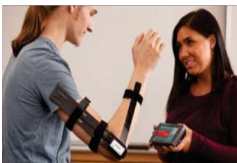
Figure 2. Students using technology as the sensors in the goniometer detect ROM from elbow flexion
