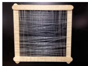
Figure 2. Sample Water Filter Design made from 8 lb. monofilament Fishing Line
