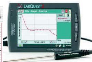
Figure 3. LabQuest 2 is an interface used to collect sensor data with its built-in graphing and analysis application.
