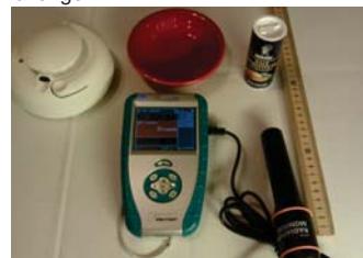
Figure 3. Radioactive source with varying distances from the monitor
