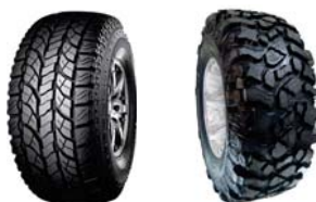
Figure 2. Tire on the left is designed for highway driving; for mud on the right.
