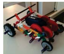
Figure 2. K'NEX Car Demonstrating Compound Gear Train
