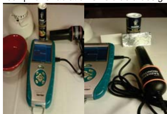
Figure 2. Radioactive sources with labquest, radiation monitor and shields
