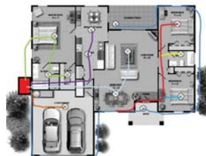
Figure 3: House wiring diagram drawn on the layout
