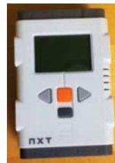
Figure 3. The Lego Mindstorm NXT 2.0 intelligent brick (cpu).
