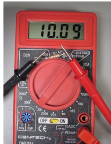
Figure 1. Voltmeter measuring a 10k Ohm resistor's actual resistance. The voltmeter reads 10.09.
