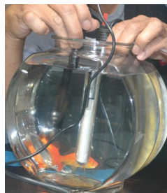
Figure 1. Experimental set-up measuring Dissolved Oxygen at high temperature in an aquarium with fish.
