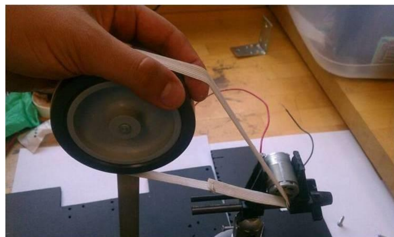
Figure 1. Image of a pulley system with an integrated motor and a voltage supply.
