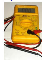
Figure 4. Multimeter- Used in this set-up to measure voltage between electrodes.
