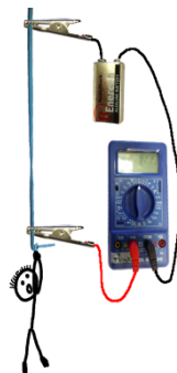
Figure 1. Stretching the rubber band results in a change in its resistance.
