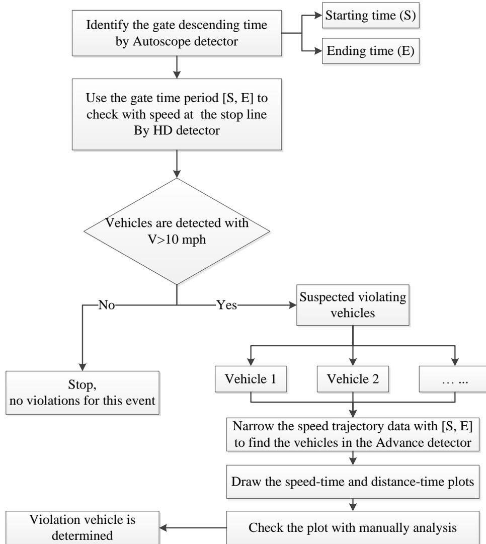
**Figure 3.6** The logic of the data synchronization
