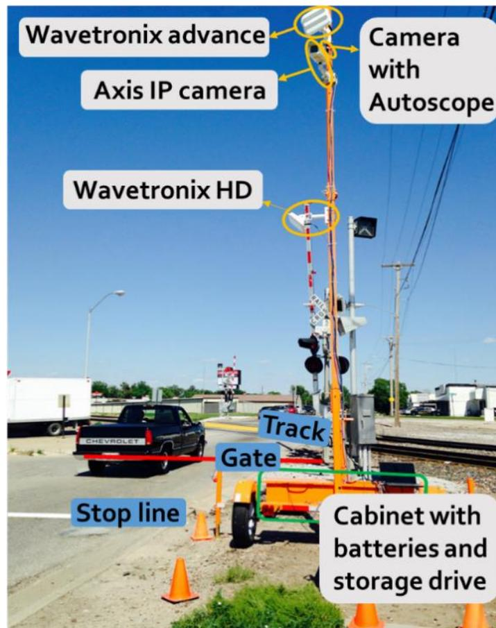
**Figure 3.2** Mobile trailer data collection (MTDC) system
