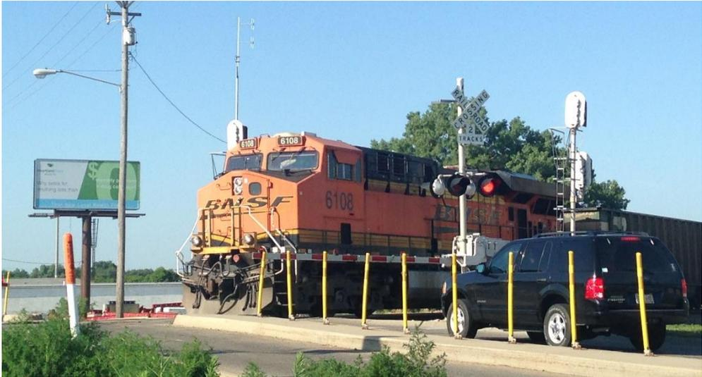
**Figure 1.2** An active HRGC equipped with red flashing beacons and automatic gate arms
