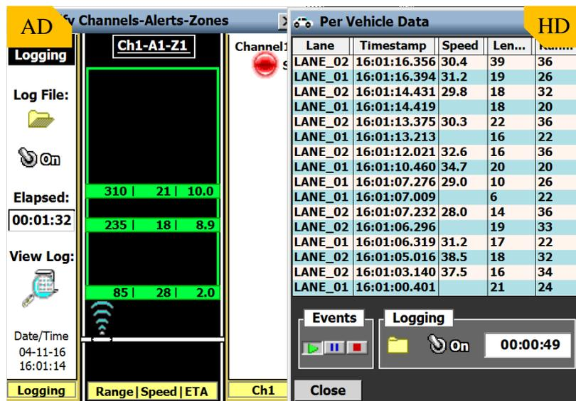
**Figure 3.3** Real-time data collection interfaces of Wavetronix AD (left) and HD (right)
