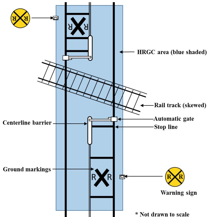
**Figure 1.3** Components of an active HRGC (Source: Figure 8B-6 in MUTCD, 2003 (10))
