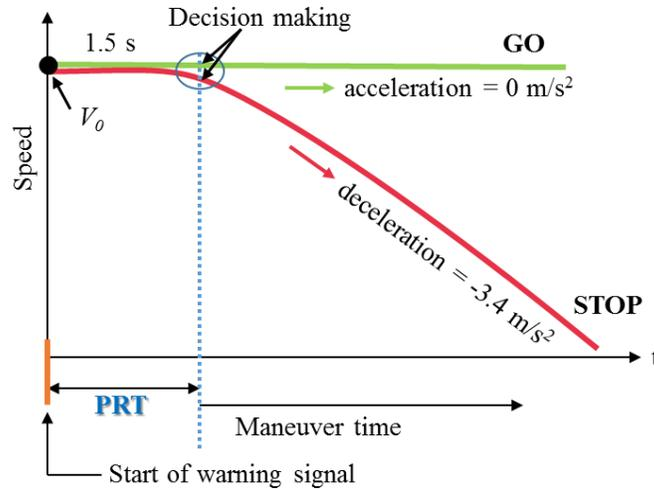
**Figure 2.2** Traditional simplistic stop/go model and the recommended values by AASHTO
