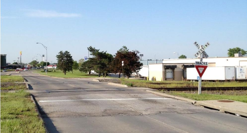
**Figure 1.1** A passive HRGC equipped with a yield sign and a crossbuck
