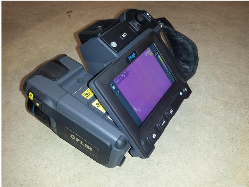
**Figure 3.1. FLIR T640 thermal camera**
