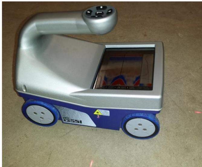
**Figure 3.2. GSSI StructureScan Mini HR GPR device**
