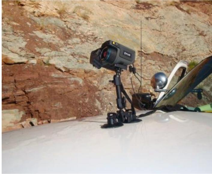
**Figure 6.3. Thermal camera set-up on high rail truck**
