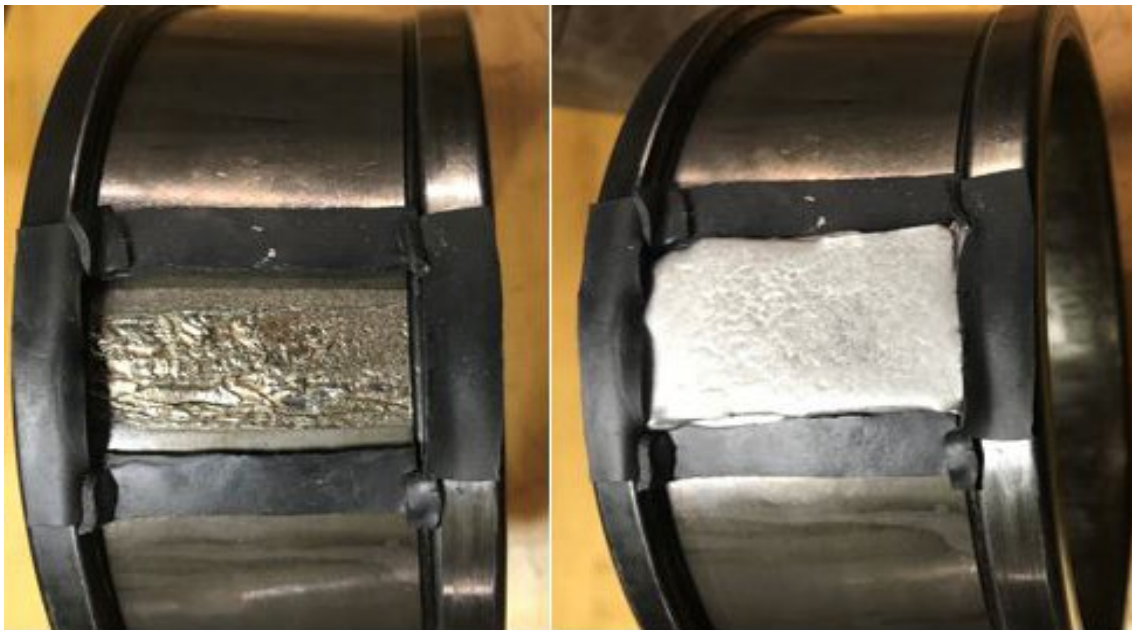
Figure 8. A picture demonstrating the casting procedure using Bismuth; (left) spalled surface outlined with tacky tape; (right) Bismuth alloy cast
