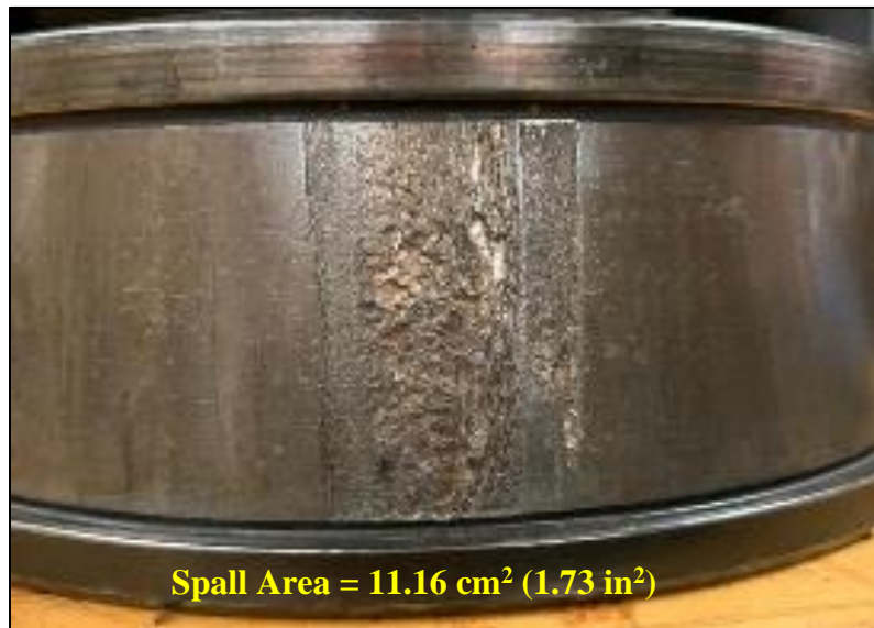
Figure 20: Cone spall– Experiment 228B
