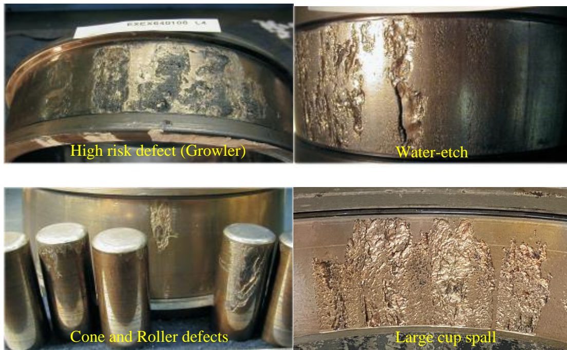
Figure 2: Tapered-roller bearing defects
