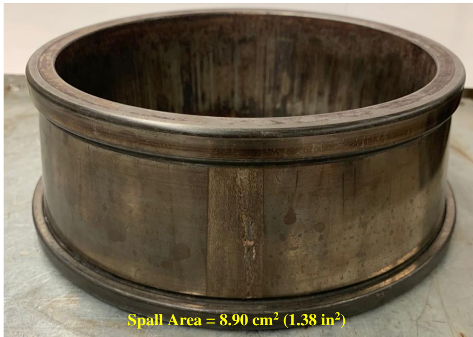
Figure 41: Experiment 233 cone defect tested in B3 position
