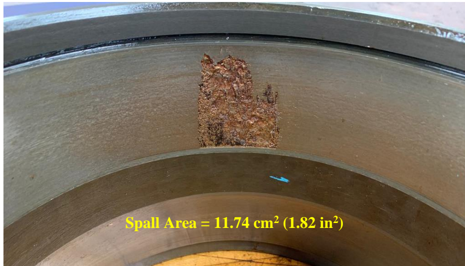
Figure 35: Experiment 231 B3 – medium-size cup spall
