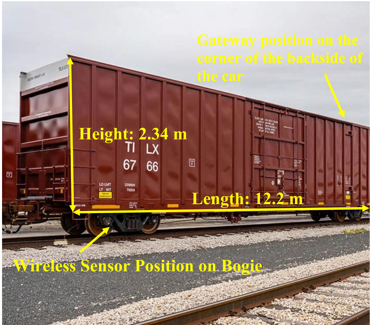
Figure 14: Boxcar with Dimensions and Sensor Placement Locations [21]
