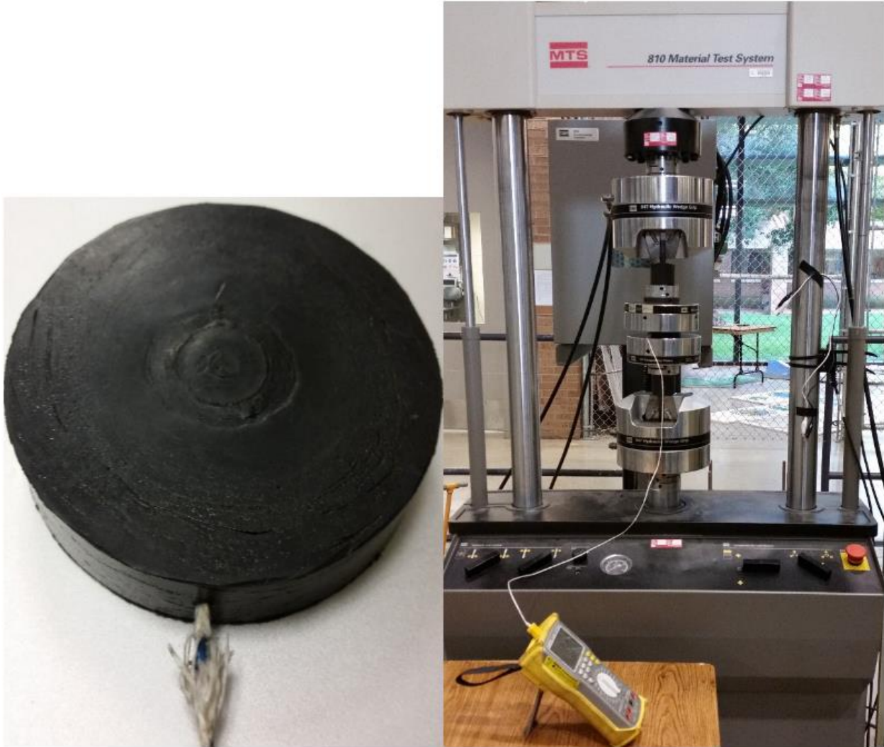
Figure 2.1. Hysteresis heating cylindrical sample of virgin pad material with thermocouple inserted in the specified location (left) and Hysteresis heating test setup on 810 Material Test System (MTS) (right).
