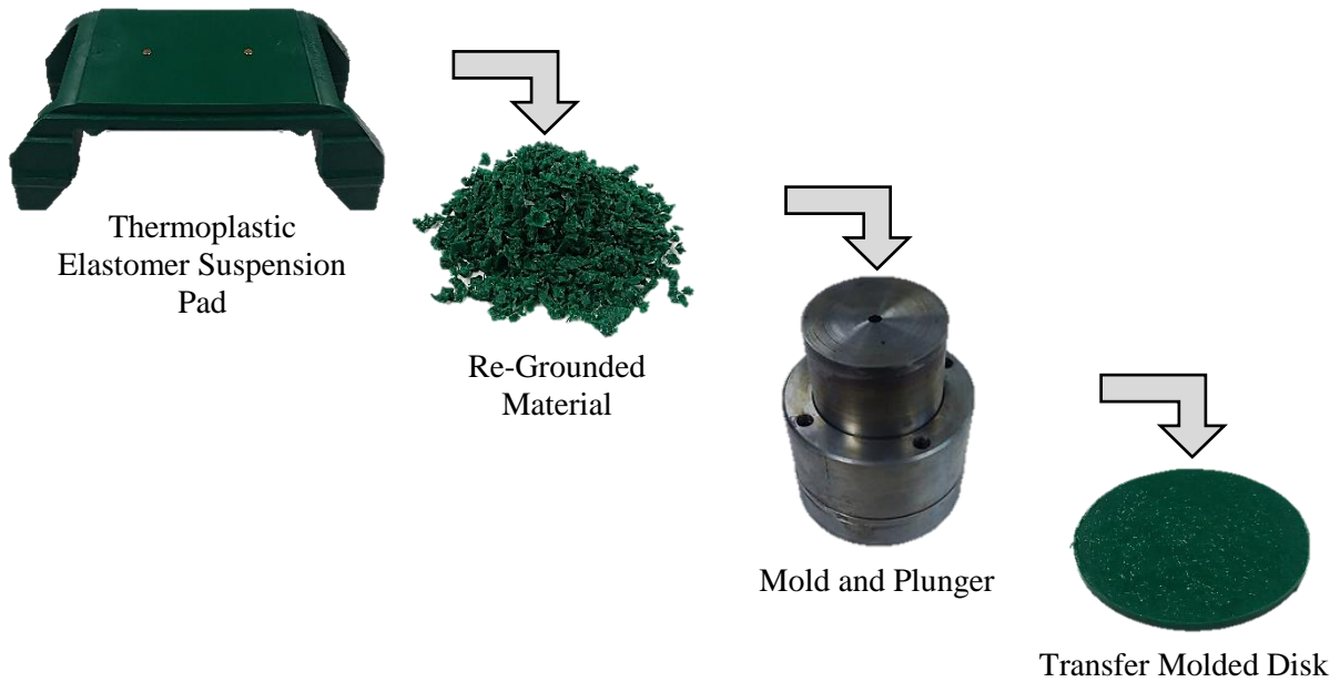
Figure 2.6. Transfer molding process for DMA sample preparation.
