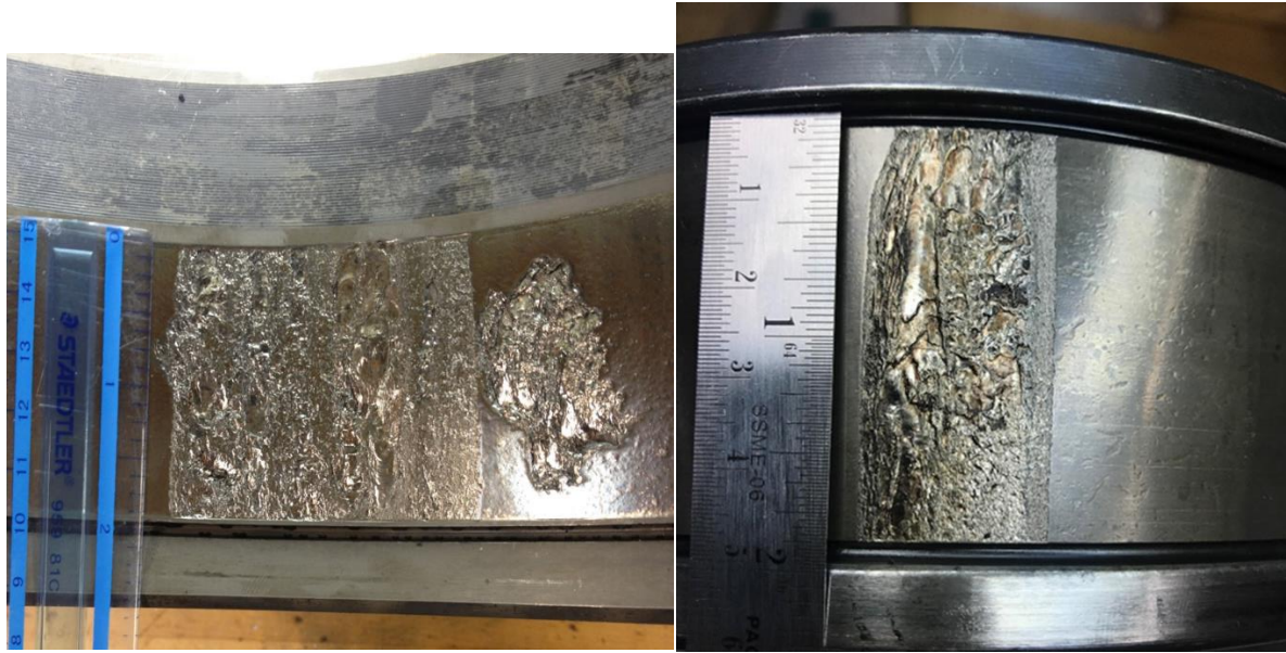
Figure 18. Outer ring (cup) spall from Exp. 198C (pictured left) and inner ring (cone) spall from Exp. 202A (pictured right)
