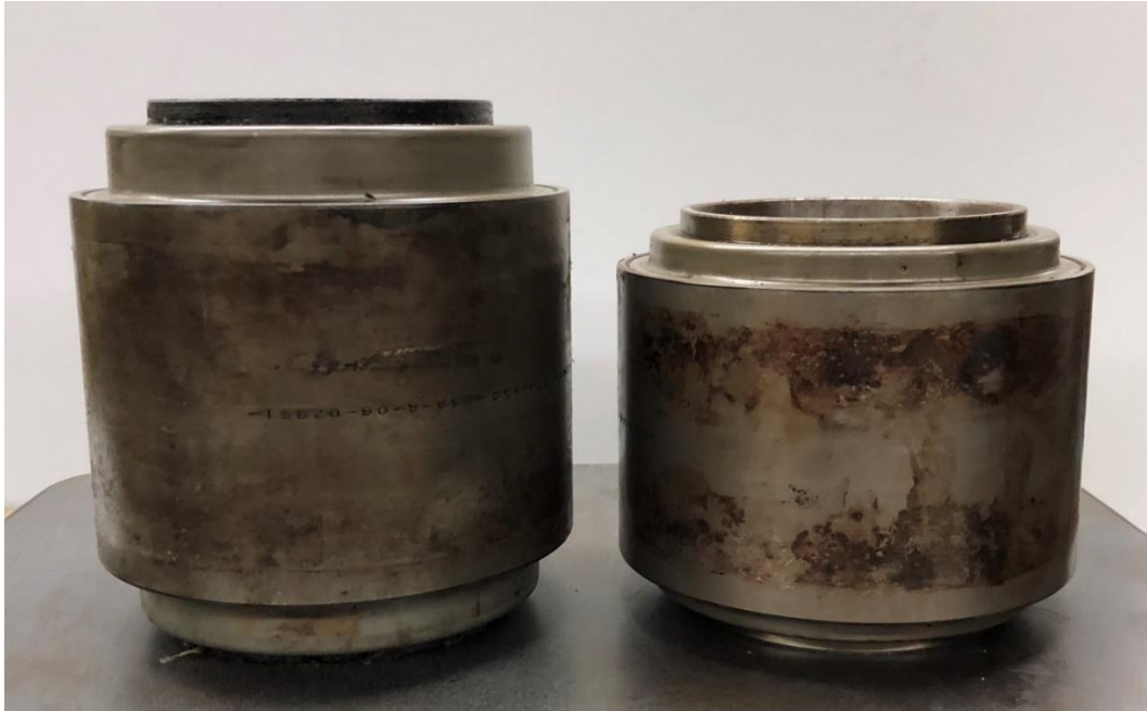
Figure 3. Class F (pictured left) and Class K (pictured right) bearings
