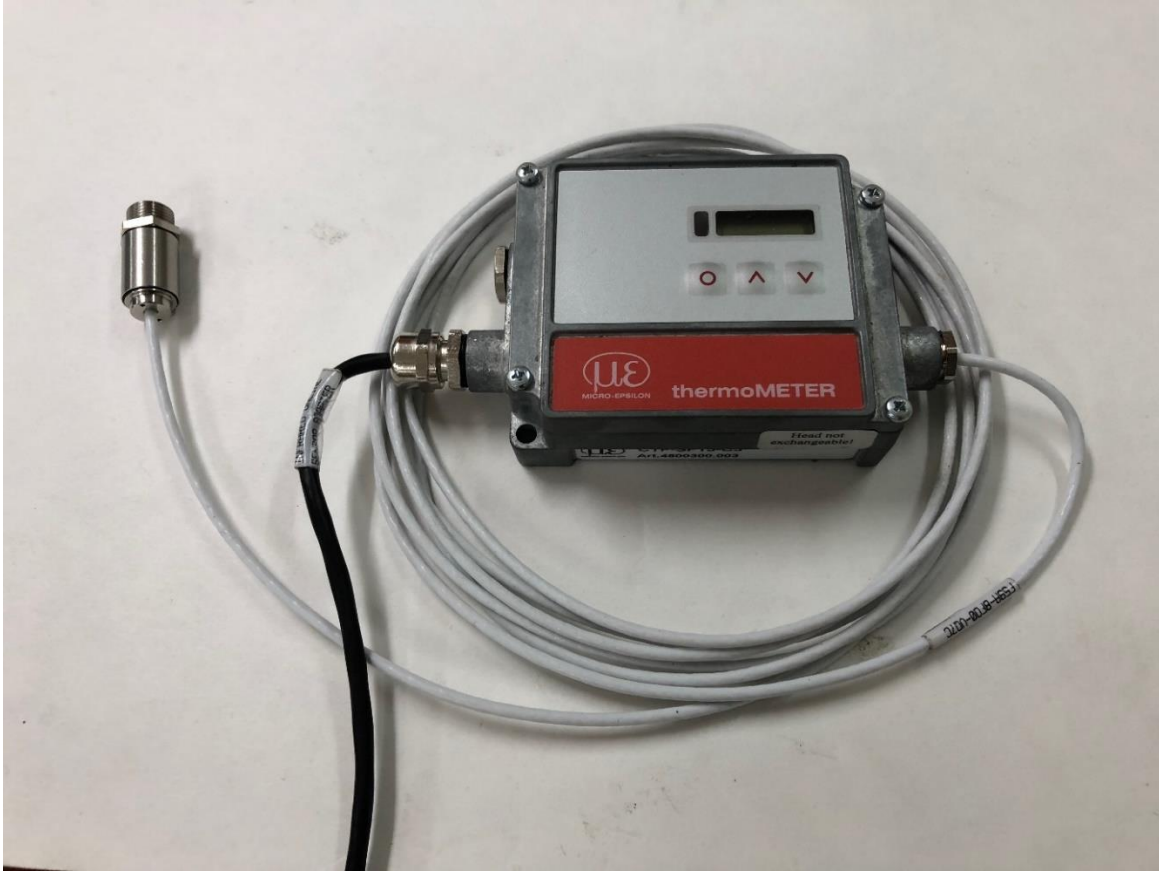
Figure 16. MICRO-EPSILON infrared (IR) temperature sensor
