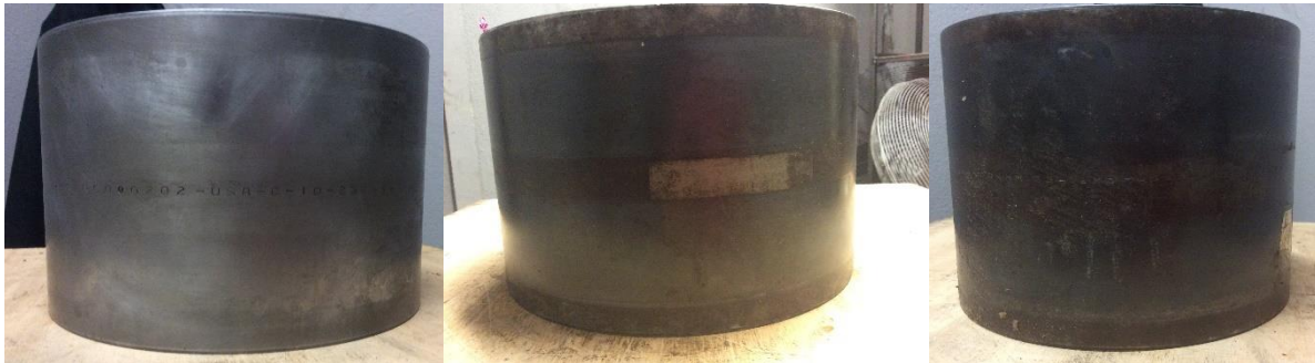
Figure 21. Examples of bearing cups used for emissivity testing includes brushed surface (left), moderately used surface (center), and heat-tinted rusted surface (right)
