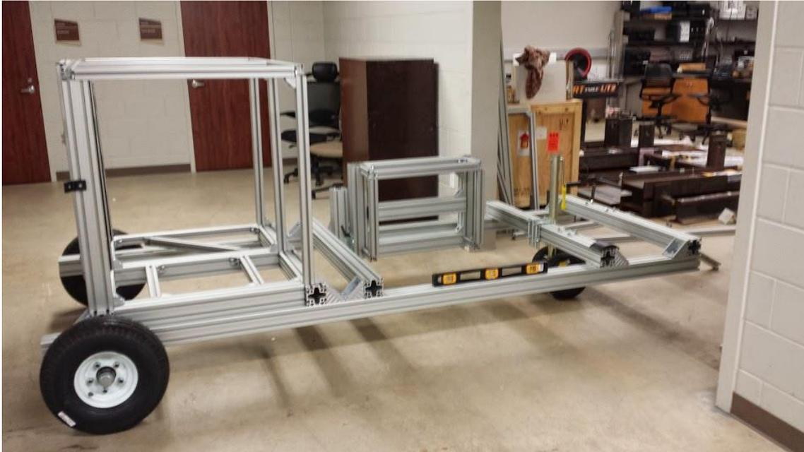
**Figure 5.16: Primary cart frame attached to the trailer axle and side mount jack.**
