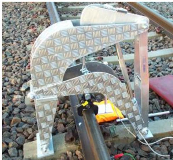
**Figure 2.3: VERSE measurement system (VERSE, 2012).**
