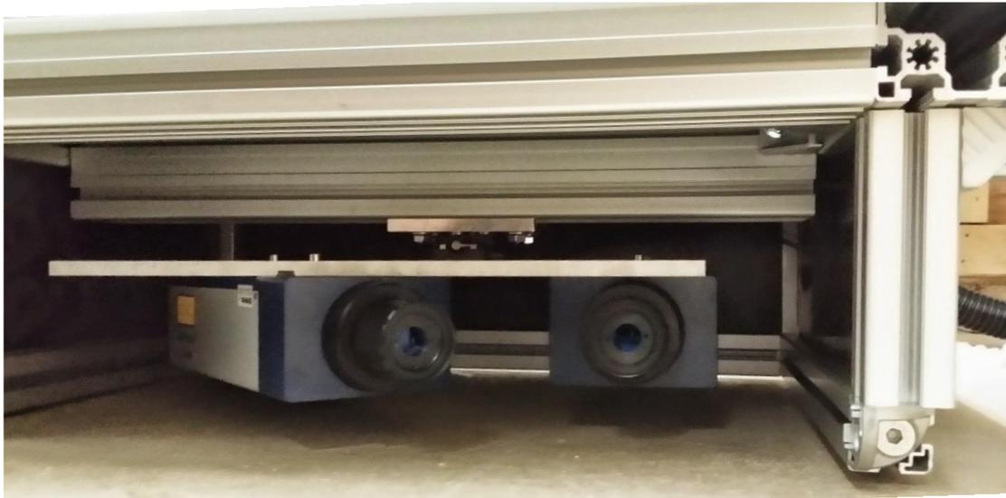
**Figure 5.17: Front view of the LDV housing unit shows the Thor MTS50 motorized translation sandwiched between the two 10 mm aluminum mounting plates.**
