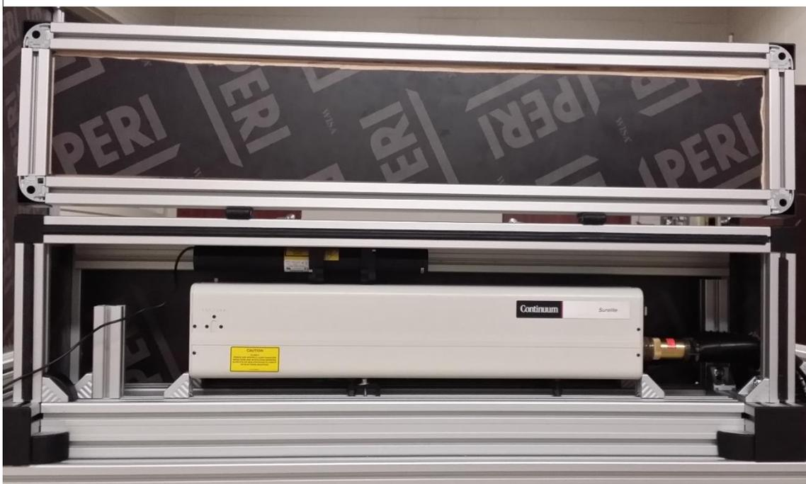
**Figure 5.18: Opened Nd:YAG housing unit.**
