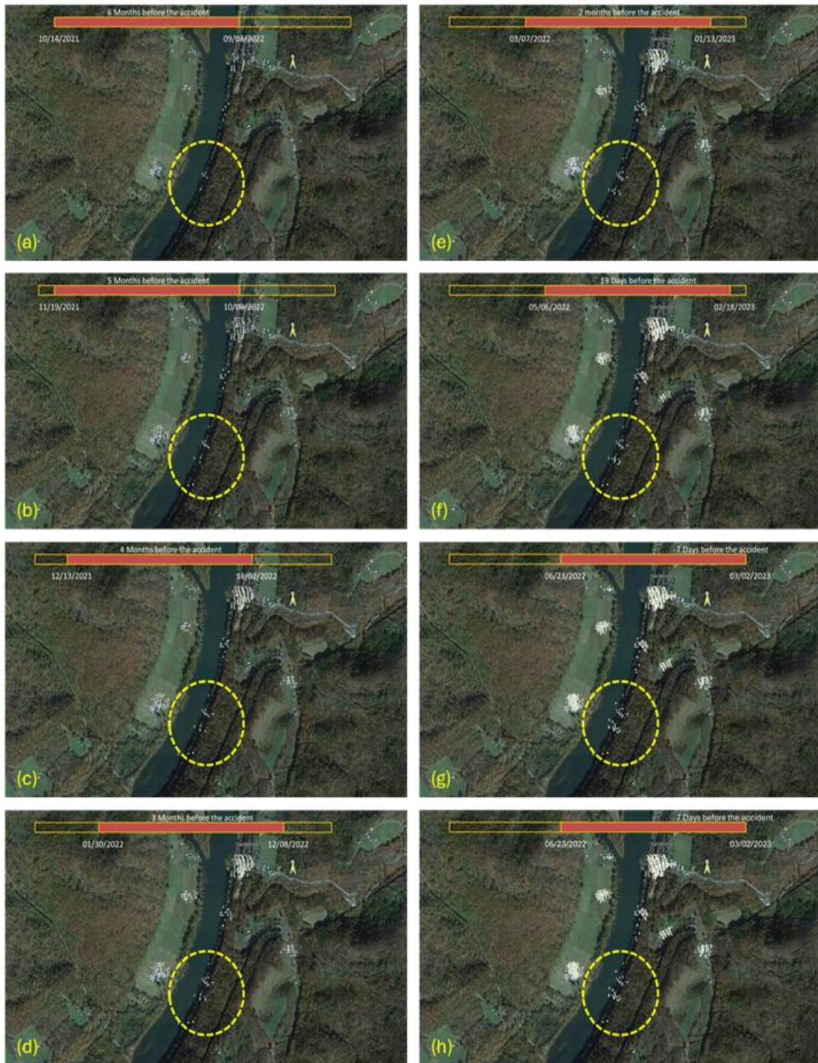
Figure A.41 DS Accumulation at (a) 6 months; (b) 5 months; (c) 4 months; (d) 3 months; (e) 2 months; (f) 1 months; (g) 19 days; and (h) 7 days before the rockfall event and derailment
