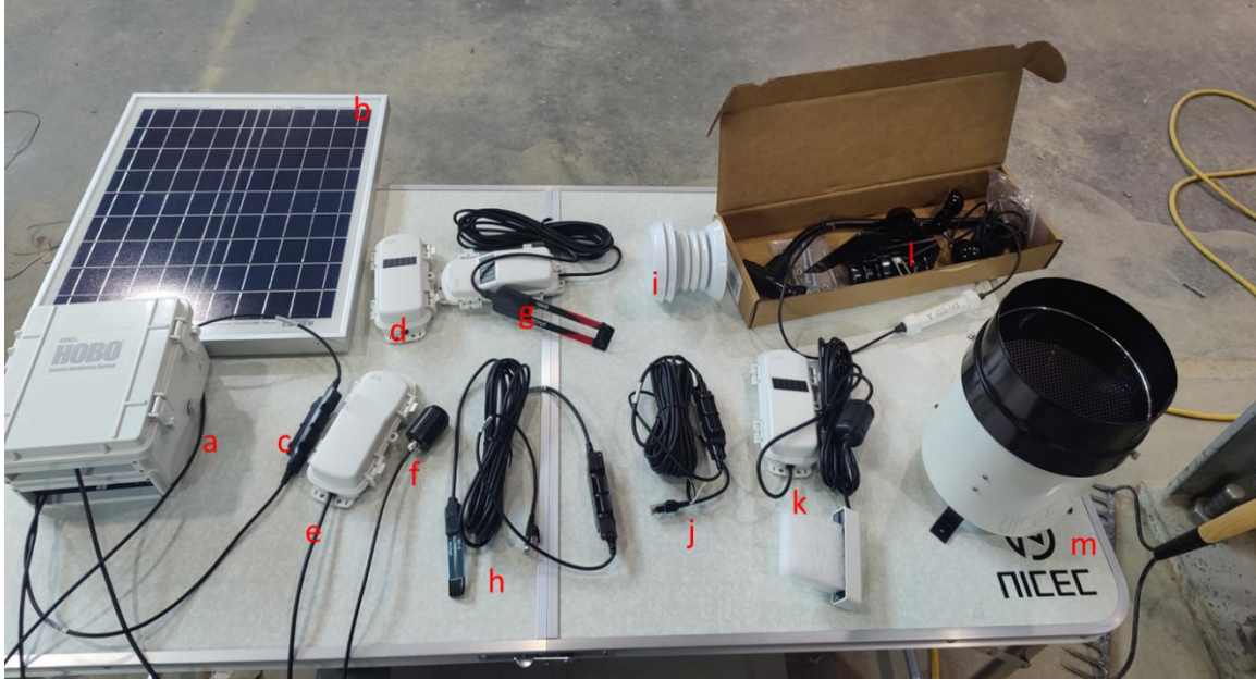
Figure B.10 The equipment deployed in the site (a) Remote Sensing Station (b) Solar panel (c) Leaf wetness smart sensor (d) Repeater (e) Modulator (f) Light Sensor (g) Soil moisture sensor (h) Soil moisture sensor (i) Solar Radiation Shield (j) Runtime Smart Sensor (k) Soil moisture (l) Davis Anemometer (m) Rain Gauge
