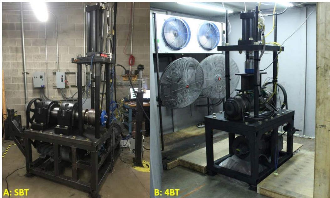
Figure 19: A) single bearing tester (SBT), and B) four bearing tester (4BT).
