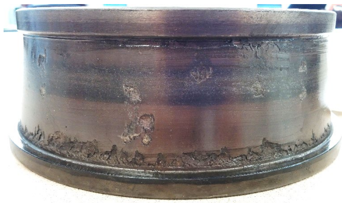
Figure 3: Water-etched bearing defect.
