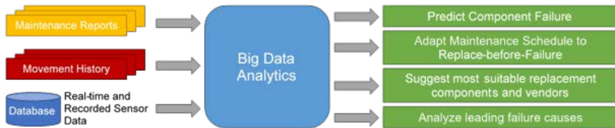
Fig 1 - Envisioned overall architecture for Big Data Analytics for Maintenance Optimization
