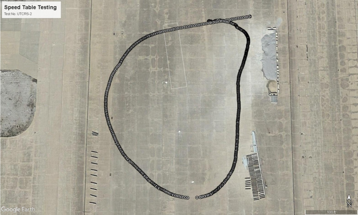
Figure 62. GPS Data Overlaid on Google Earth Image of the Test Site, Test No. UTCRS-2
