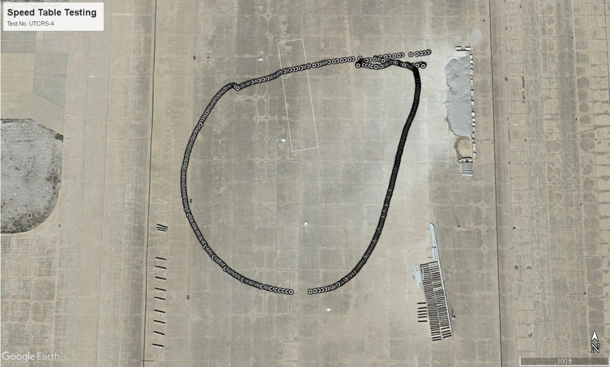
Figure 68. GPS Data Overlaid on Google Earth Image of the Test Site, Test No. UTCRS-4
