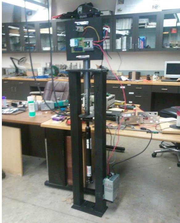
Figure 4: Hydraulic pressure control system for vertical loading
