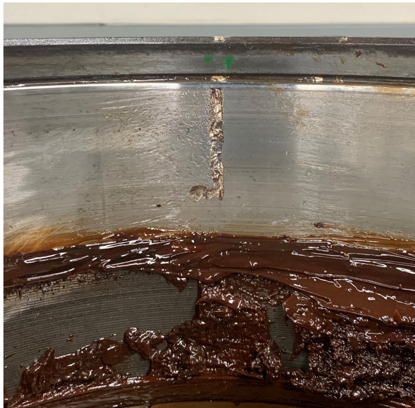
Figure 8. Post-test condition of the bottom raceway of MxV6 after spall formation.
