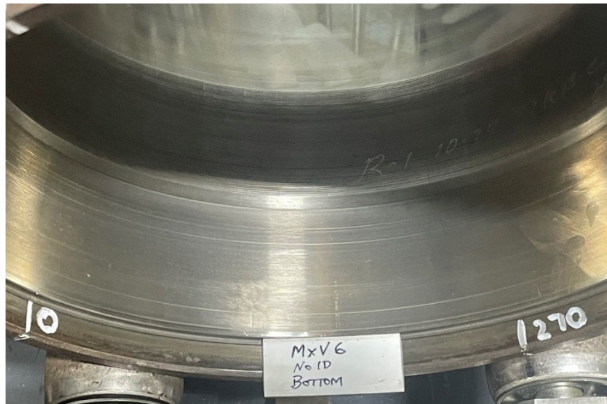
Figure 7. Pre-test condition of the bottom raceway of MxV6.
