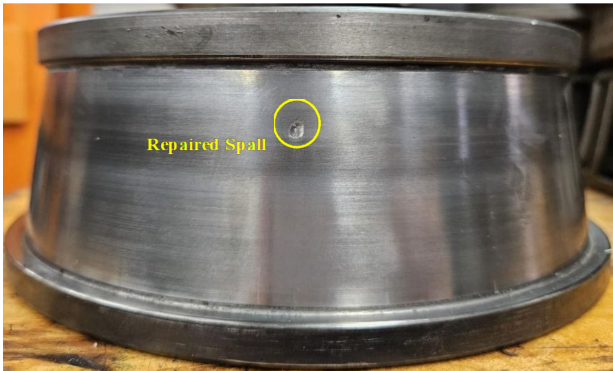
Figure 19: L4 IB cone raceway showing repaired spall region
