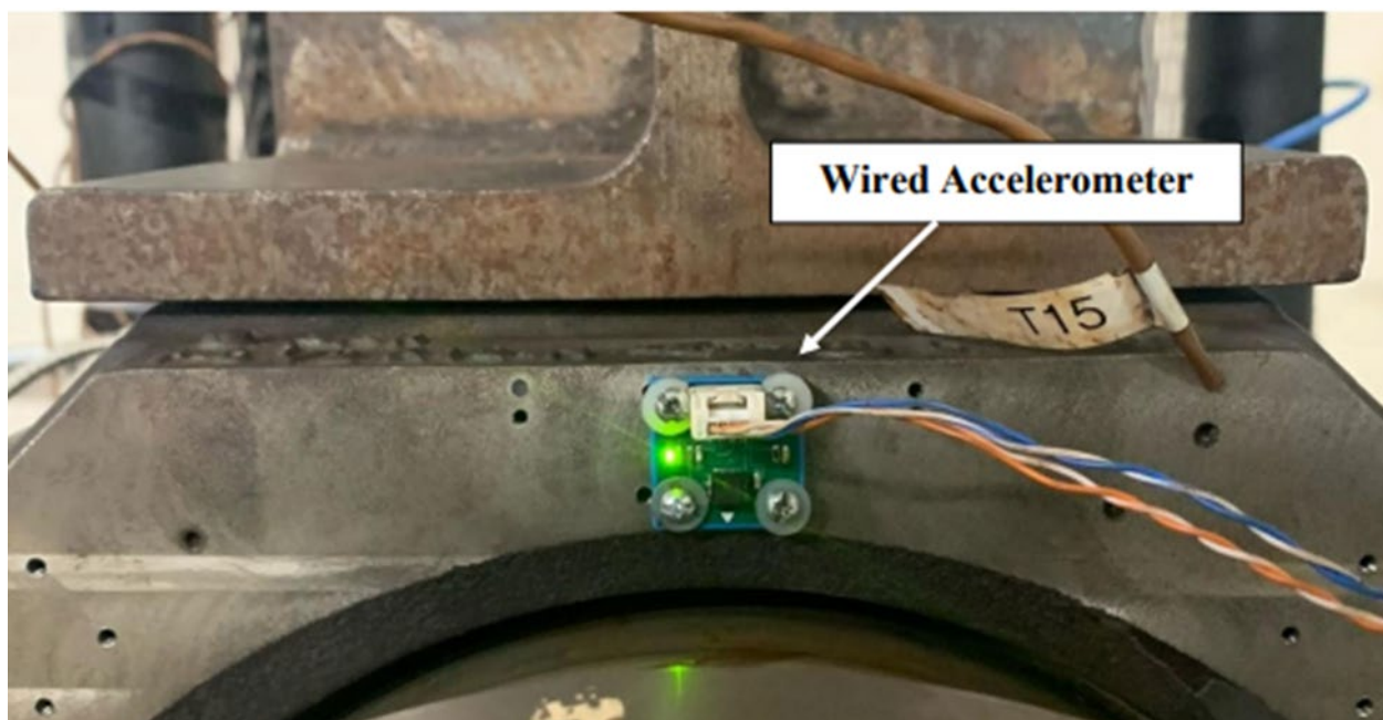
Figure 4: Wired accelerometer location in the top-dead-center (TDC) position
