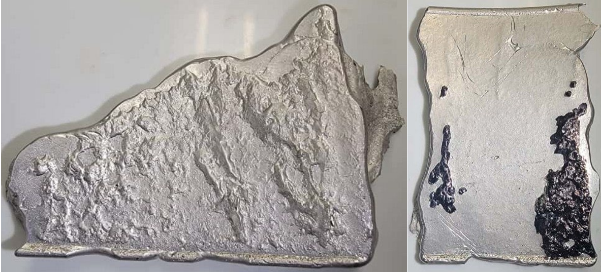
Figure 85: B2 (12-Month) bearing OB cone spall with an area of 2.03 in 2 (13.10 cm 2 ) (left) and 0.42 in 2 (2.71 cm 2 ) (right)
