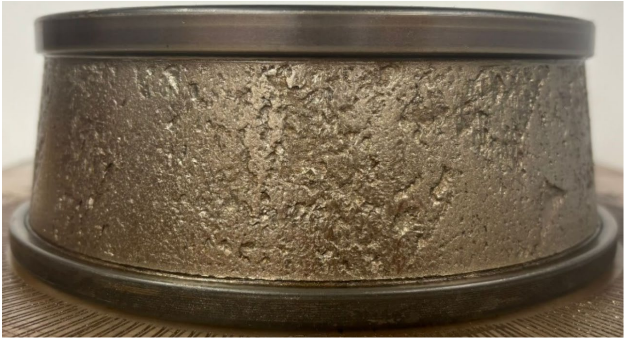
Figure 66: B2 (12-Month) bearing OB cone raceway – Picture 1
