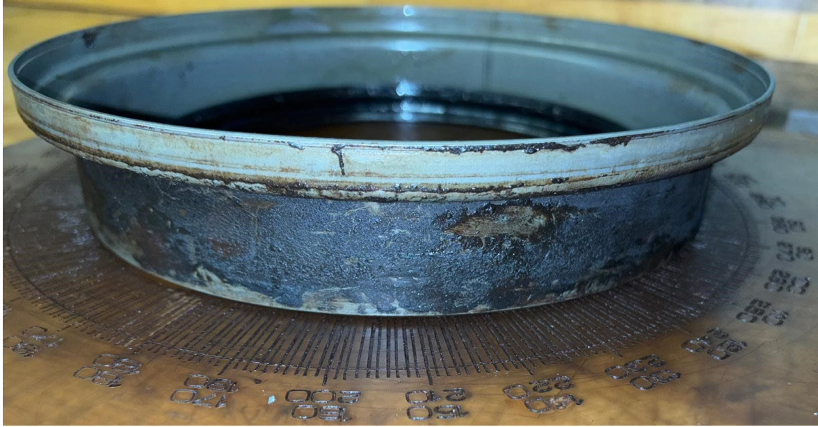
Figure 103: Grease leak area of Bearing R2 IB seal
