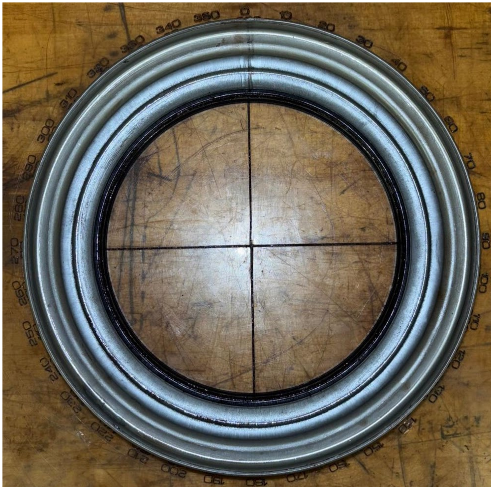
Figure 104: Overview of Bearing R2 OB seal
