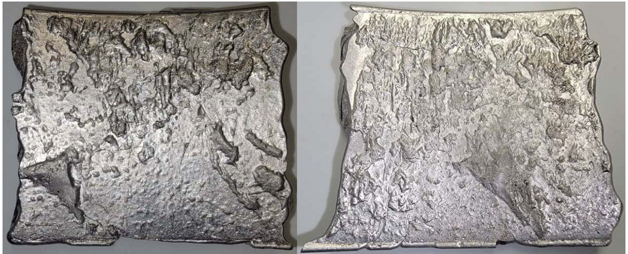
Figure 84: B2 (12-Month) bearing OB cone spall with an area of 4.41 in 2 (28.45 cm 2 ) (left) and 4.27 in 2 (27.55 cm 2 ) (right)
