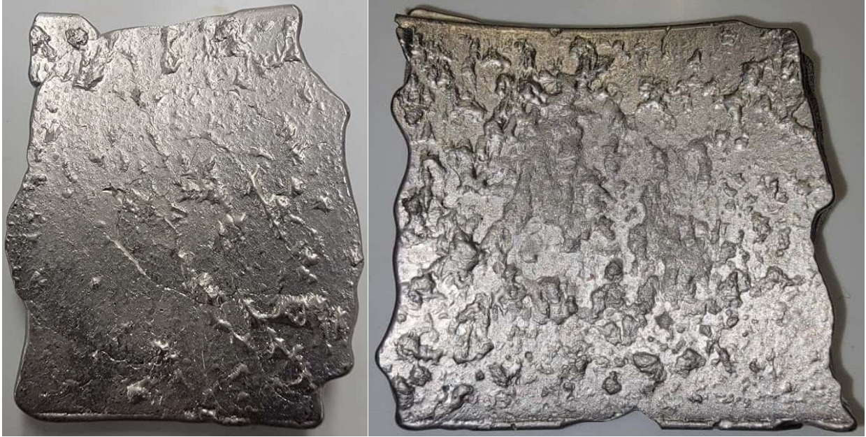
Figure 83: B2 (12-Month) bearing OB cone spall with an area of 3.12 in 2 (20.13 cm 2 ) (left) and 3.96 in 2 (25.55 cm 2 ) (right)
