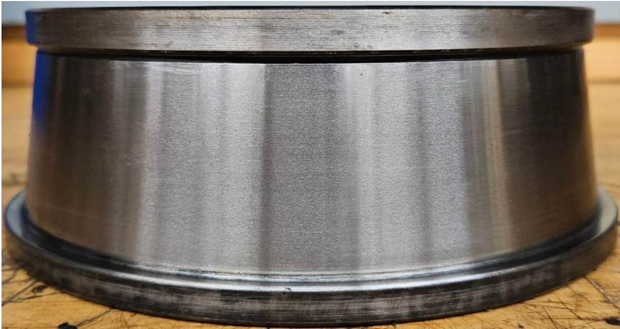
Figure 14: R4 outboard (OB) cone raceway
