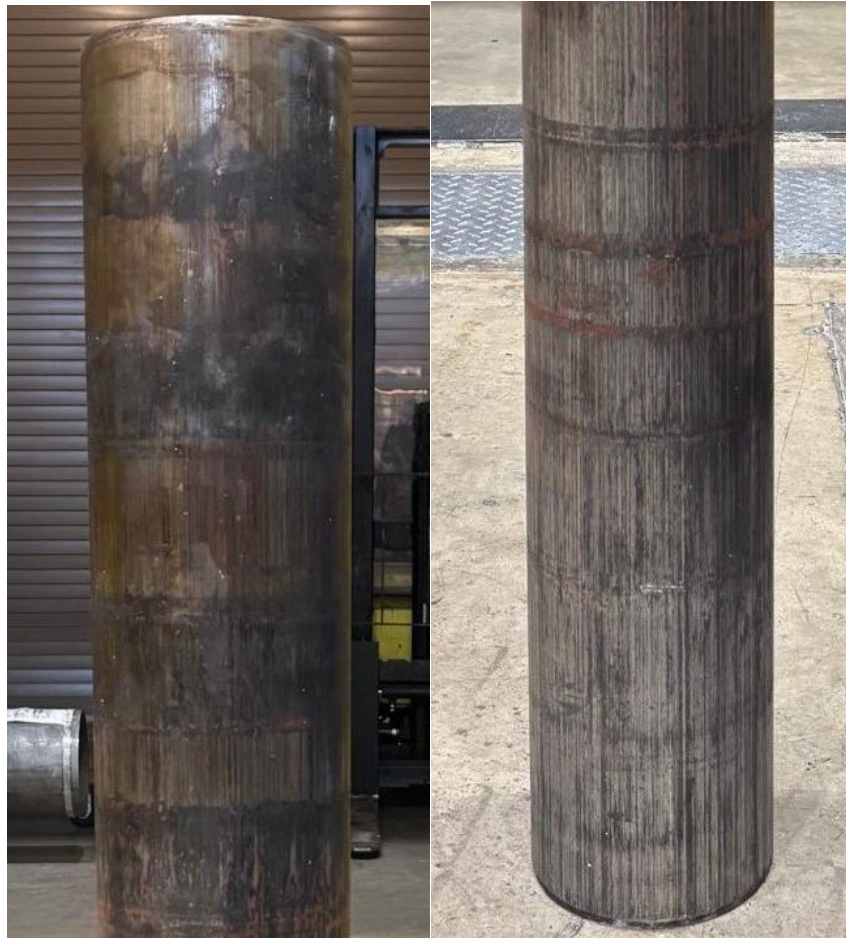
Figure 97: Test axle post-press-off
