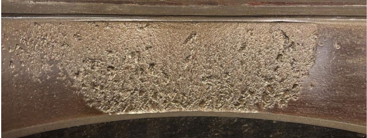
Figure 79: B2 (12-Month) bearing cup OB raceway on unloaded side (270°)
