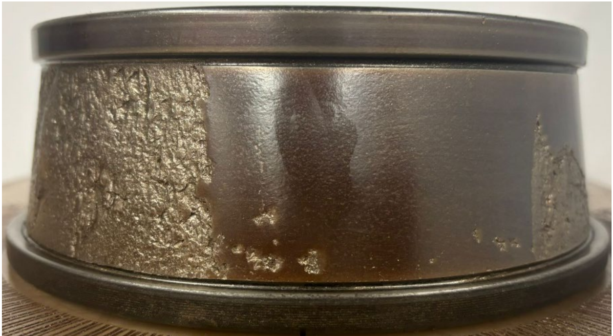
Figure 67: B2 (12-Month) bearing OB cone raceway – Picture 2
