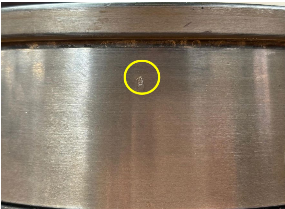
Figure 44: Small spall (0.015 mm 2 / 0.006 in 2 ) on R2 IB cone raceway
