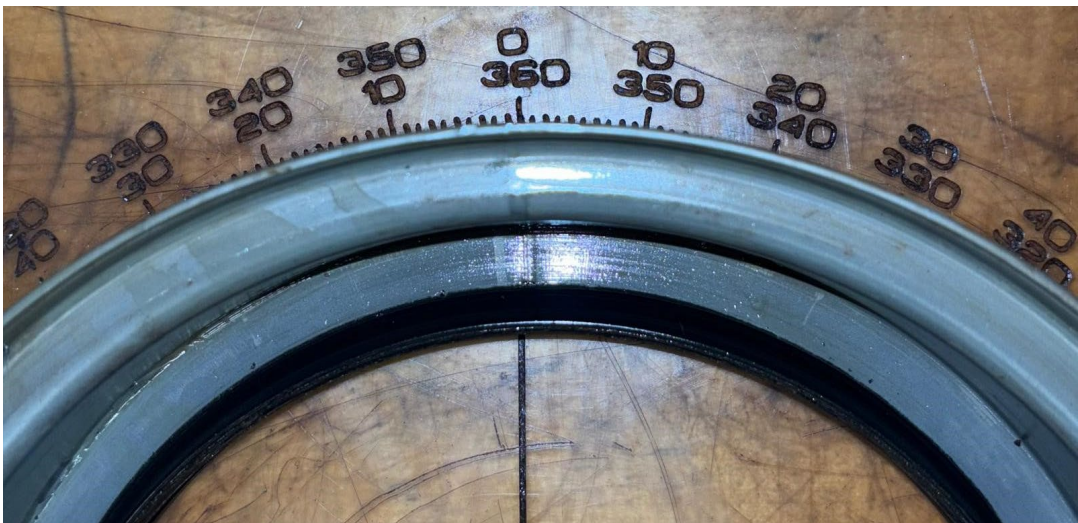
Figure 102: Seal weld line of Bearing R2 IB seal
