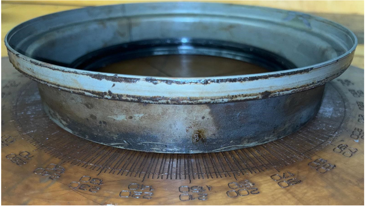
Figure 100: Grease leak area of Bearing L2 OB seal
