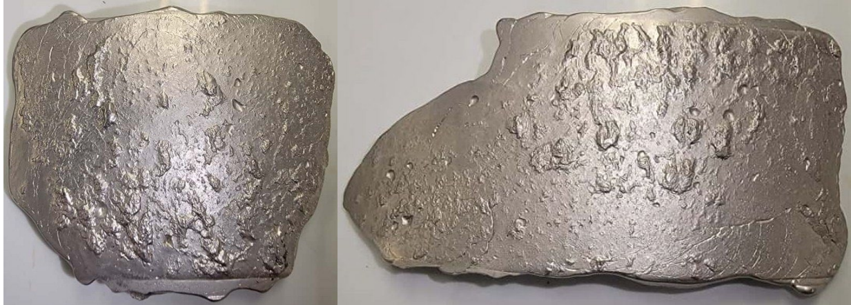
Figure 81: B2 (12-Month) bearing OB cup spall with an area of 4.57 in 2 (29.48 cm 2 ) (left) and 7.31 in 2 (47.16 cm 2 ) (right)
