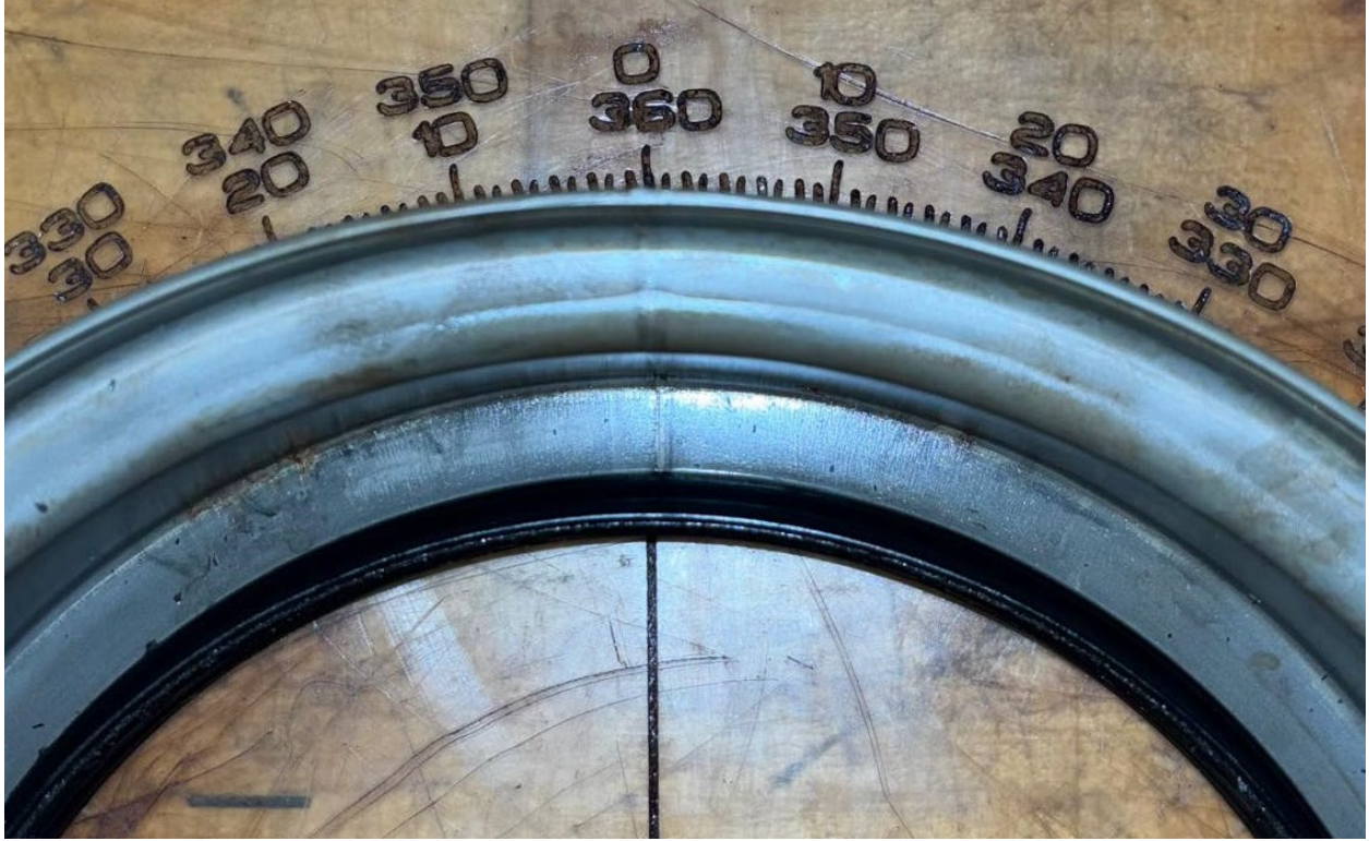
Figure 99: Seal weld line of Bearing L2 OB seal
