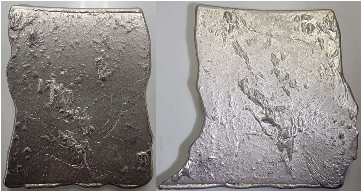
Figure 82: B2 (12-Month) bearing OB cone spall with an area of 3.18 in 2 (20.52 cm 2 ) (left) and 3.32 in 2 (21.42 cm 2 ) (right)
