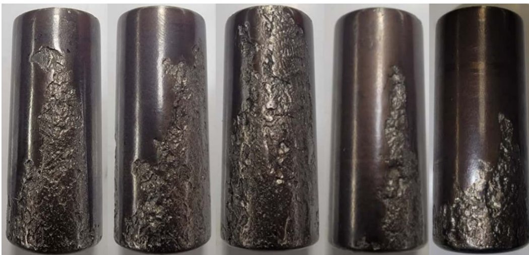
Figure 86: B2 (12-Month) bearing OB cone assembly roller spalls with areas of 1.30 in 2 (8.39 cm 2 ), 1.45 in 2 (9.35 cm 2 ), 2.41 in 2 (15.55 cm 2 ), 0.84 in 2 (5.42 cm 2 ), and 1.07 in 2 (6.90 cm 2 ) [left to right]
