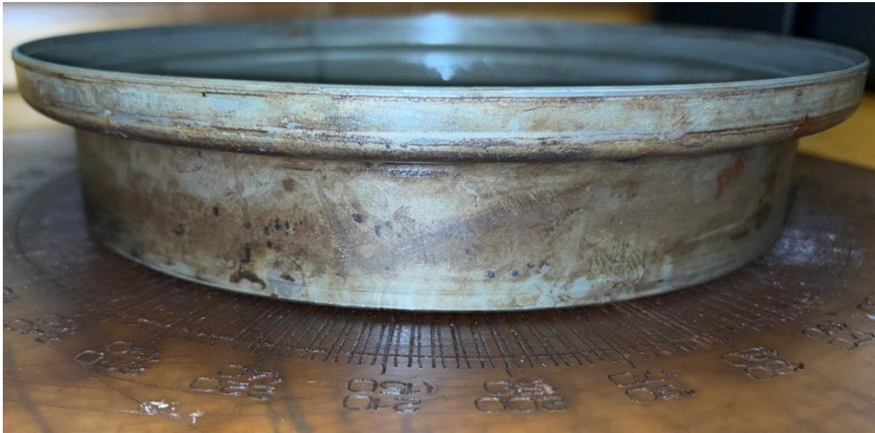
Figure 106: Grease leak area of Bearing R2 OB seal
