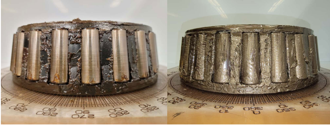
Figure 107: Comparison of the IB cone assembly (left) and OB cone assembly (right) for the B2 (12-Month) bearing
