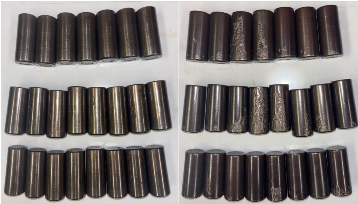
Figure 80: B2 (12-Month) bearing IB cone rollers (left) and OB cone rollers (right)
