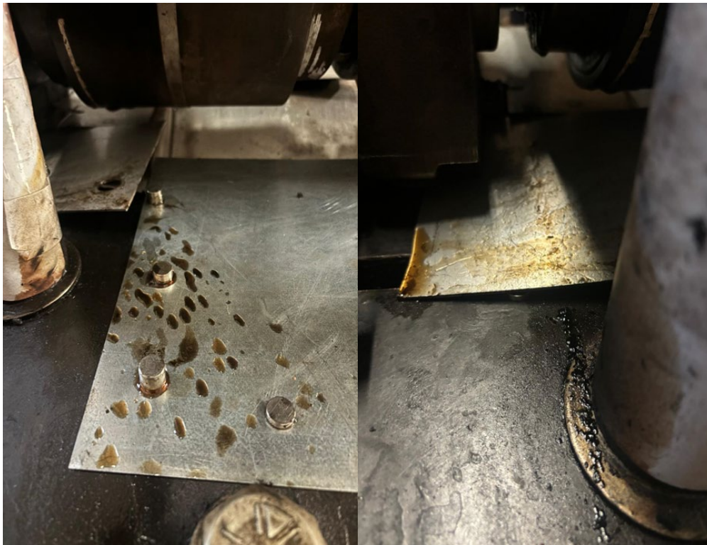
Figure 11: Pictures of grease accumulation on IB side of bearing L4
