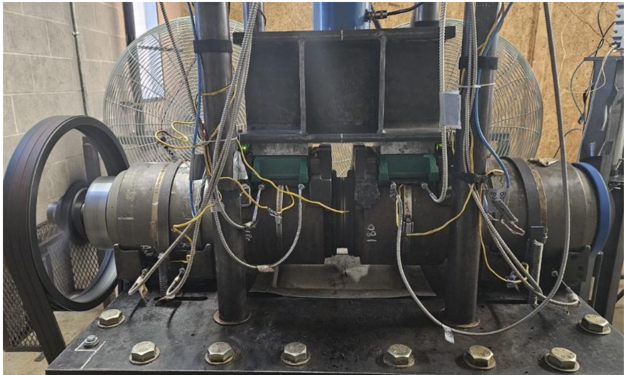
Figure 2: Picture of the UTRGV-UTCRS four bearing tester (4BT) used for this testing
