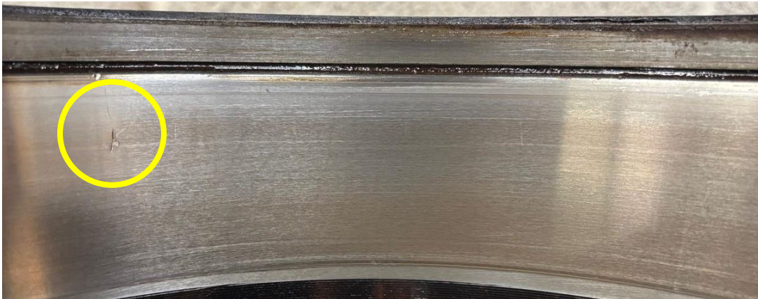
Figure 57: L2 cup OB raceway on loaded side showing a small pit on the raceway
