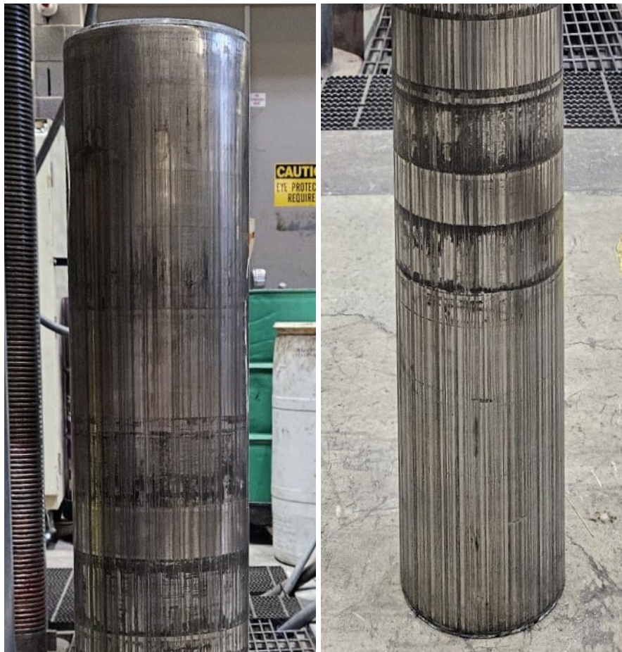
Figure 27: Test axle post press-off
