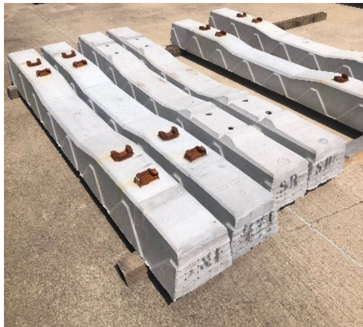
Figure 39. Concrete Crosstie at Texas A&M for Testing.
