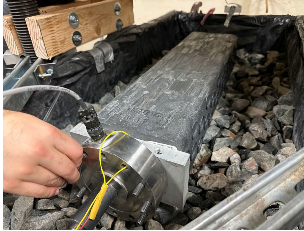
Figure 41. Wear on HDPE Crosstie.
