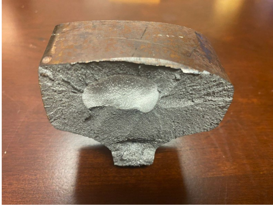
Figure 1. Railheads with internal flaws.
