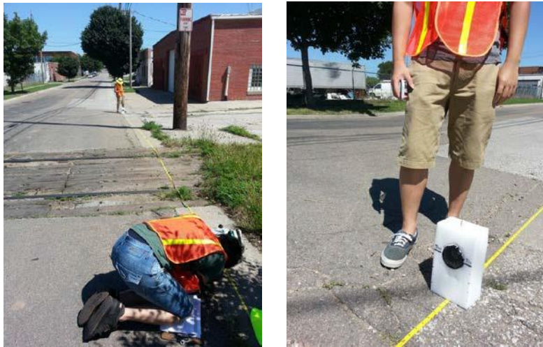
Figure 4.5 Field validation of crossing suitability using a line laser and a retro-reflective lens
