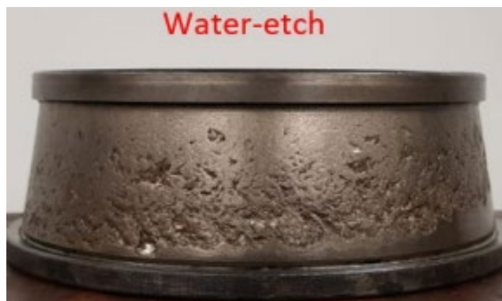
Figure 4. Water-etch damage on a cone raceway of a tapered roller bearing [3]
