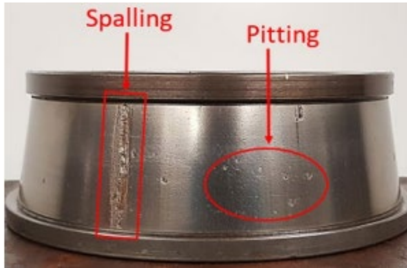
Figure 3. Fatigue spalling and pitting on a cone raceway of a tapered roller bearing [3]
