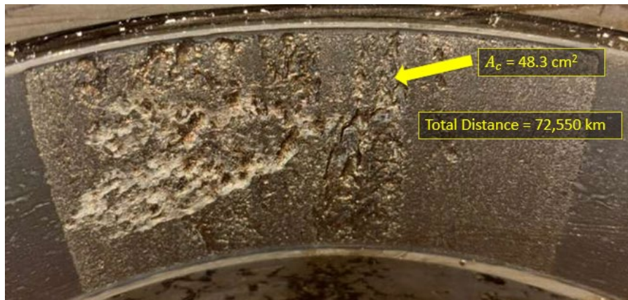
Figure 35. Post-test of the defective cup used with an OB spall
