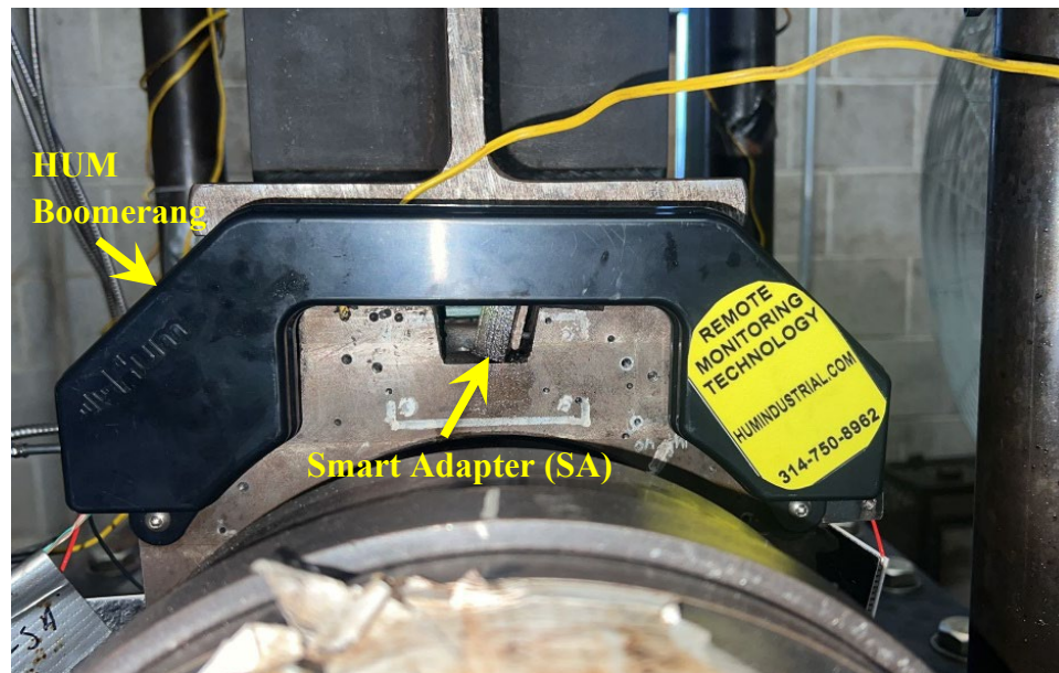
Figure 3: HUM Boomerang and UTCRS Smart Adapter accelerometer setup
