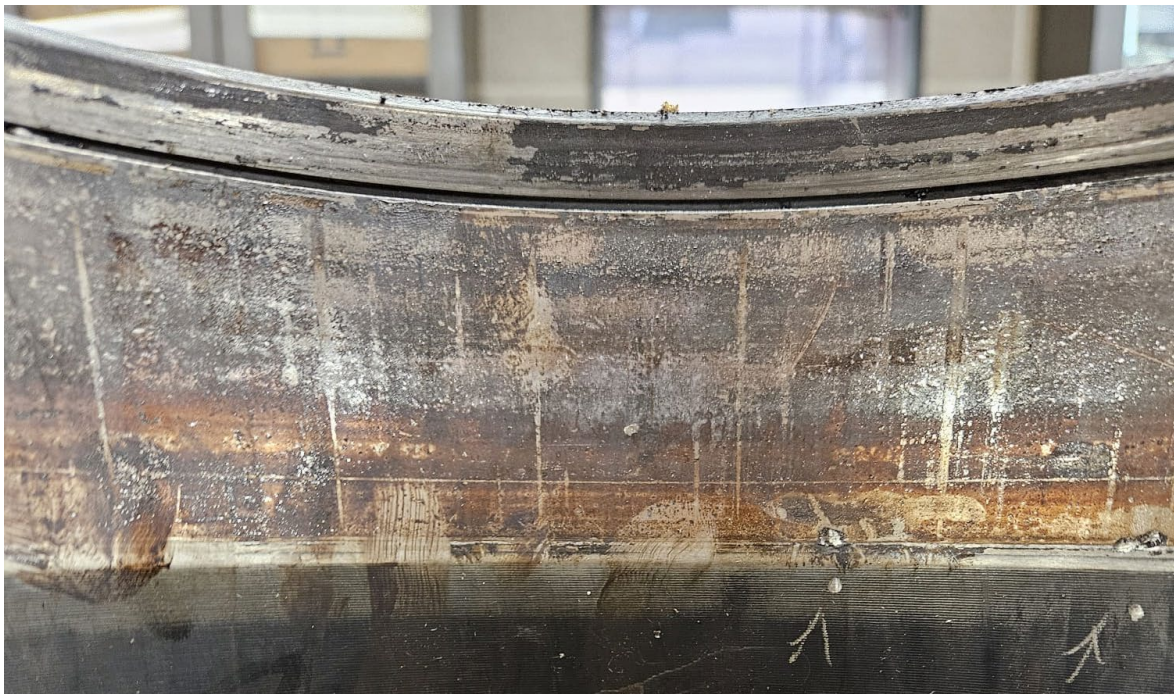
Figure 20: R7 cup (outer ring) inboard raceway on loaded side showing repaired spalls
