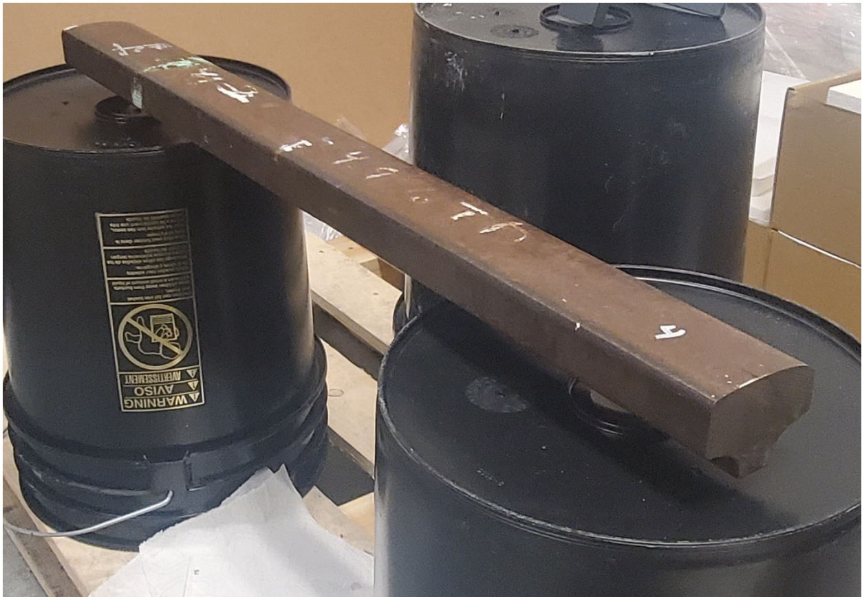
Figure 3: The fourth rail after removing the railhead for testing in the MTS machine
