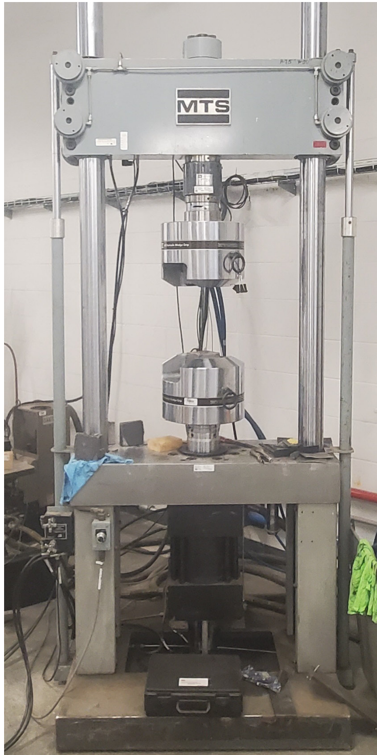
Figure 4: The 100 Kip MTS Machine to be utilized for the cyclic fatigue testing of the railhead shown in Fig. 3
