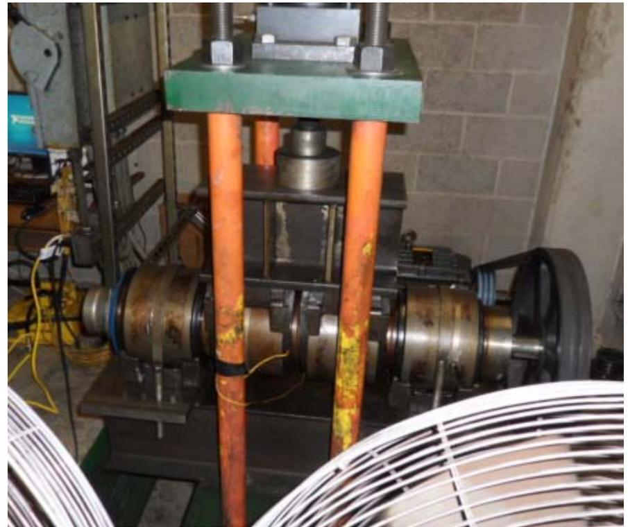
Figure 5: Photograph of the dynamic bearing tester used to conduct the service life test for this study
