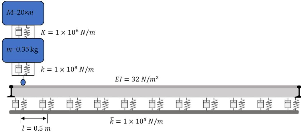
**Figure 1: Schematic of auxiliary mass system over track**
