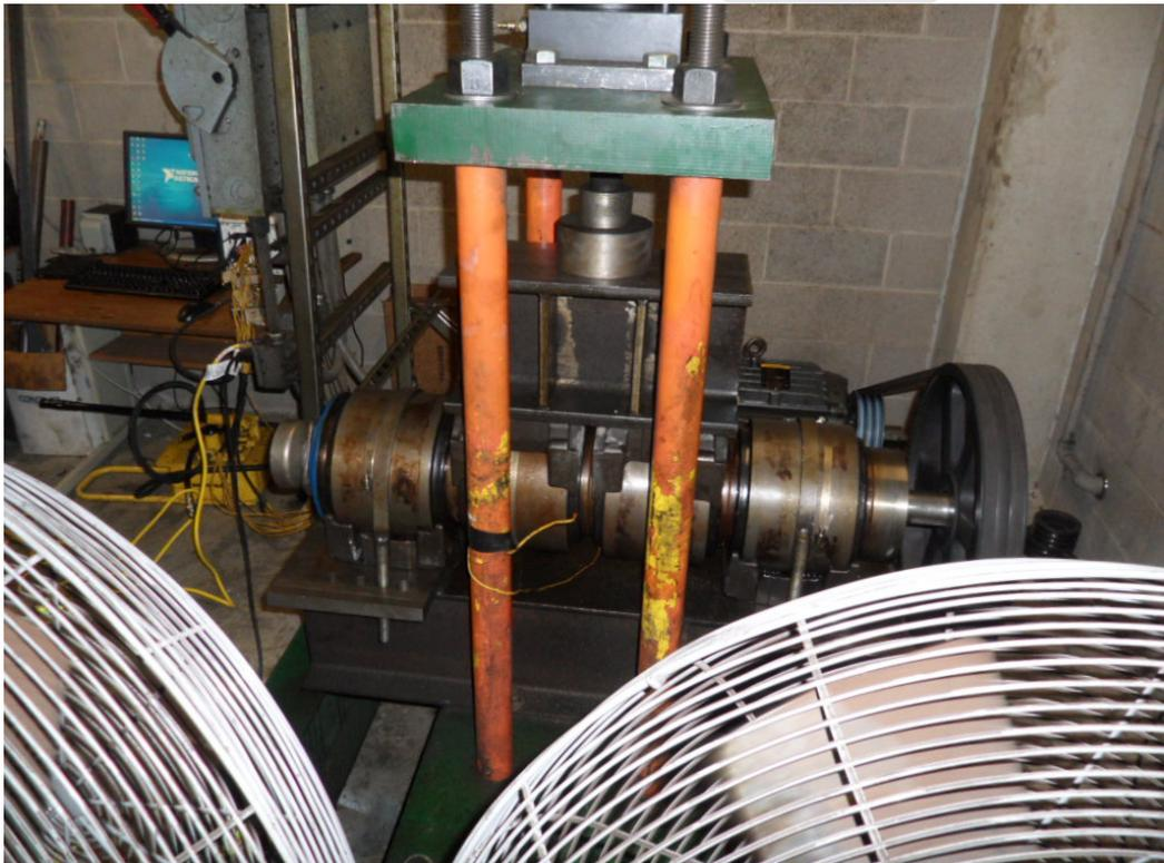
Figure 4: Photograph of the dynamic bearing tester used to conduct the service life test for this study
