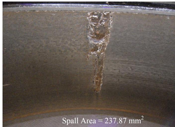
Figure 9: Photograph of the cup spall on Bearing 2 (Test Cup C) after deterioration – Teardown 2
