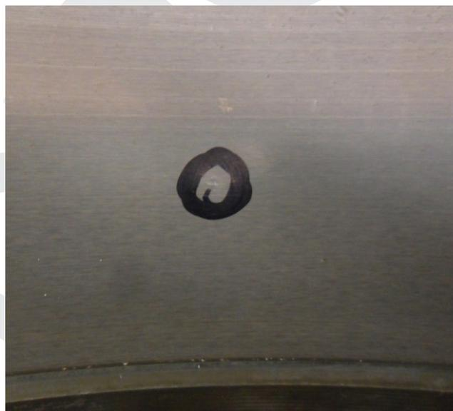
Figure 13: Photograph of the initial stage of cup spall formation on Bearing 3 (Test Cup B) – Teardown 4
