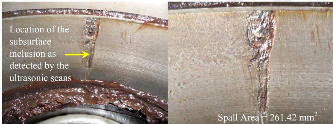
Figure 11: Photographs of the cup spall on Bearing 2 (Test Cup C) after second sign of deterioration – Teardown 3
