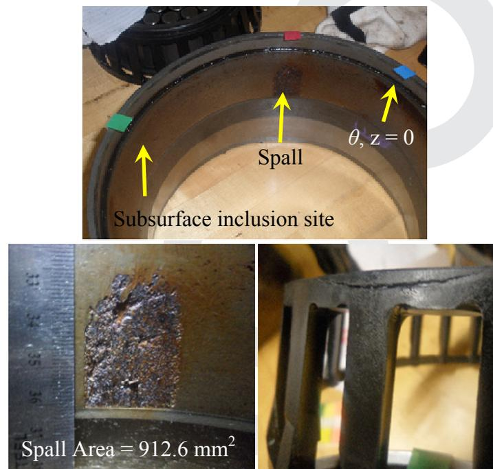
Figure 17: Pictures of the cup spall that developed on Bearing 4 (Test Cup A) and the associated cage damage – Teardown 5
