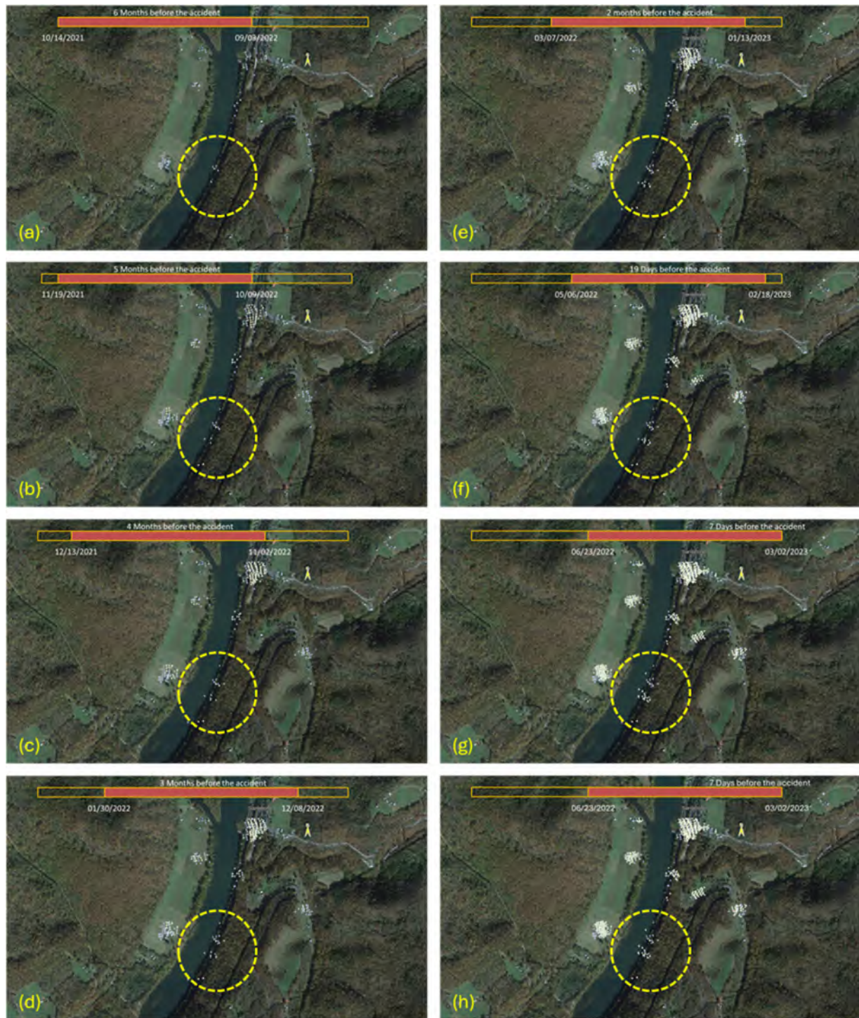
Figure 14. Validation study—DS accumulation at: (a) 6 months; (b) 5 months; (c) 4 months; (d) 3 months; (e) 2 months; (f) 1 month; (g) 19 days; and (h) 7 days before the rockfall event and derailment. Note: DS = distributed scatterers.
