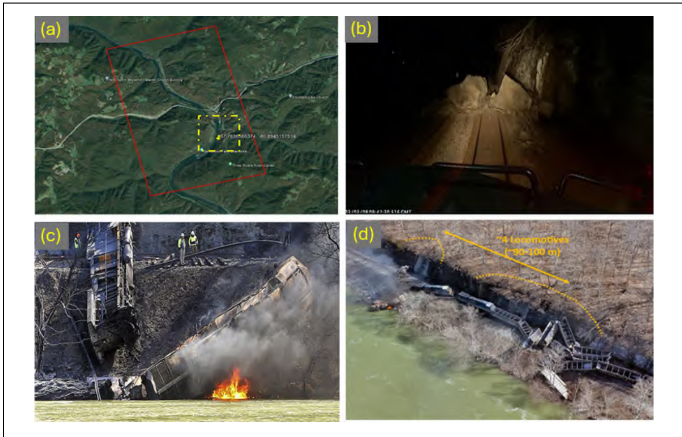
Figure 13. Validation study site: (a) incident site, (b) derailment, (c) locomotive view of rockfall, and (d) two distinct slope failures ~100 m apart.
