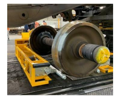
....Freight trains need an exchange of Wheel-Axle Assemblies for every 500,000 miles as well.
