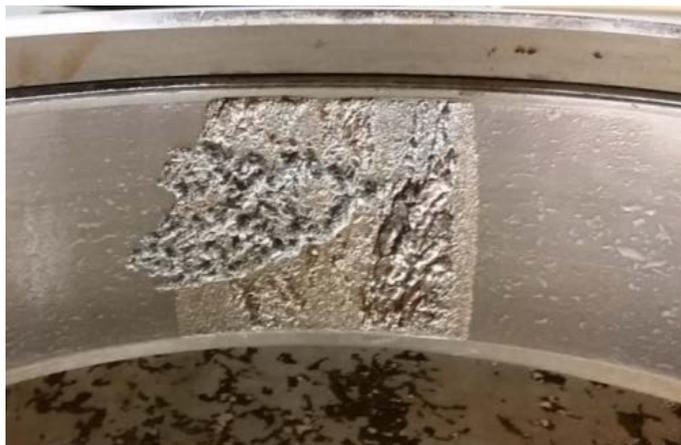
Figure 16. Photograph of Bearing R2 outer ring (cup) defect
