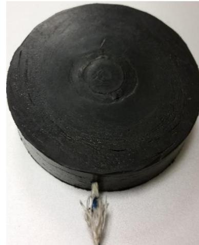
Figure 2. Hysteresis heating cylindrical specimen with thermocouple.
