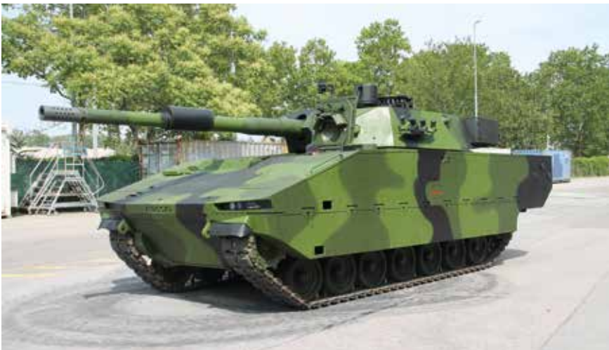
The ASCOD MMBT is based on an ASCOD platform fitted with the Leonardo Defense Systems HITFACT 120 turret armed with a 120 mm manually loaded smoothbore gun.
