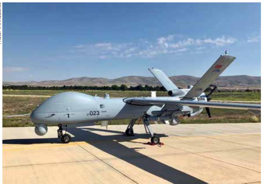
By modifying the wing surfaces, ANKA-S can take 50% more payload and operate for up to 24 hours at altitudes of 35-40,000 ft.
