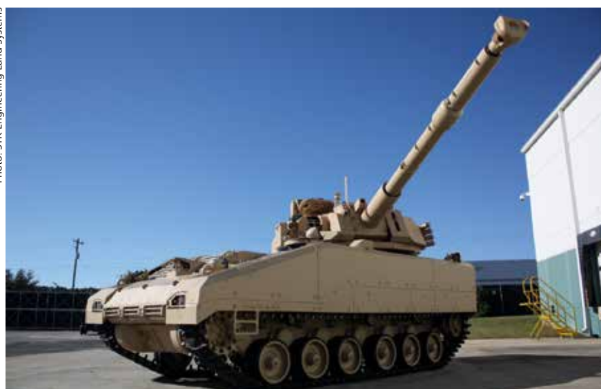
The HUNTER Fire Support Variant integrates the STK Engineering Land Systems HUNTER platform with the John Cockerill Defense C3015 two-person turret.
