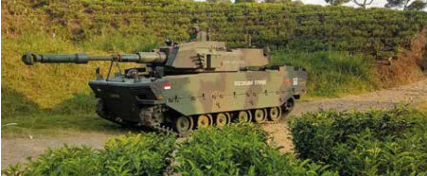
TIGER (HARIMAU) MT has been developed to meet the operational requirements of Indonesia and is fitted with a John Cockerill Defense C3105 turret armed with a 105 mm high pressure rifled gun fed by an automatic loader.
