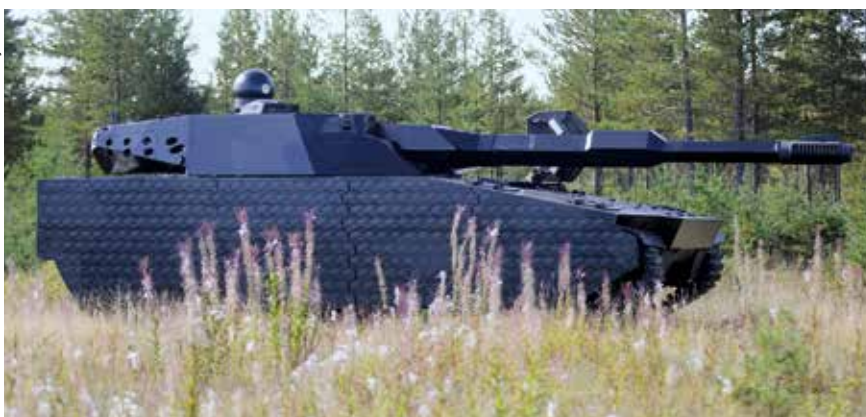
BAE Systems Hägglunds CV 90120-T armed with a Rheinmetall 120 mm smoothbore gun and fitted with adaptive signature reduction package for trial purposes.
