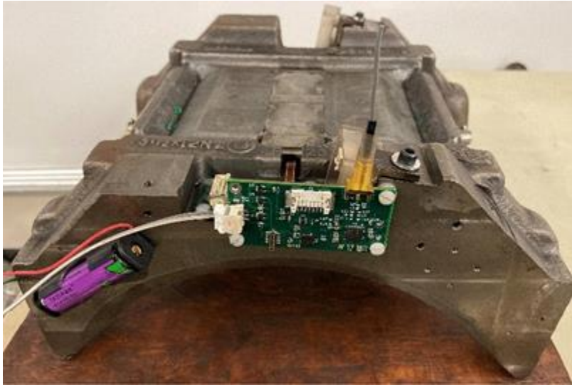
Figure 8: Wireless Onboard Condition Monitoring System powered by a battery pack [6]
