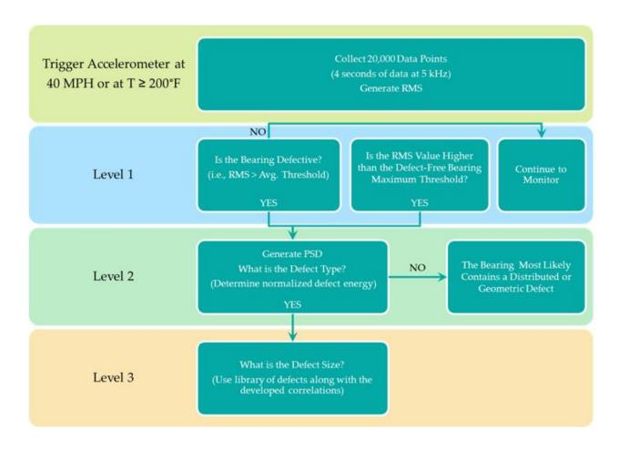
Figure 8: Defect Detection Algorithm (Montalvo, 2019)
