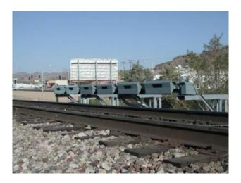
Figure 2: Trackside Acoustic Detector Systems (TADS<sup>TM</sup>)(Stewart, Flynn, Marquis, & Sharma & Associates, 2019).
