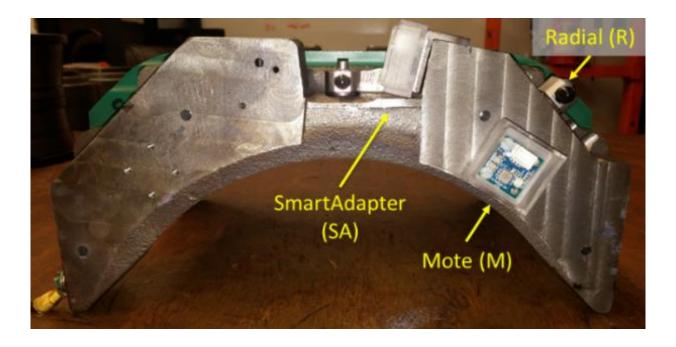
Figure 15: Bearing adapter showing accelerometer locations (Montalvo, 2019).
