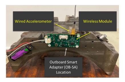
Figure 6: UTCRS Wireless Onboard Sensor Module (Cuanang, 2020).
