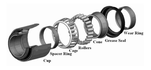
Figure 1: Detailed view of a tapered roller bearing (Hernandez, 2020)
