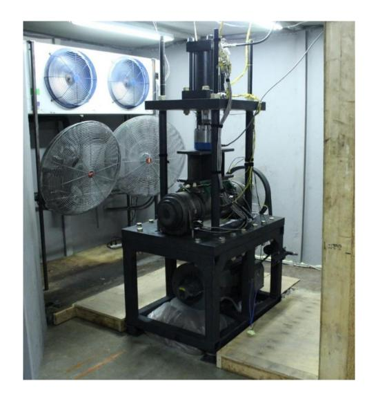
Figure 13: Four-Bearing Test Rig (4BT) (Montalvo, 2019).
