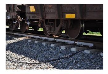
Figure 3: Wheel Impact Load Detectors (WILDs)(LBFoster, n.d.).
