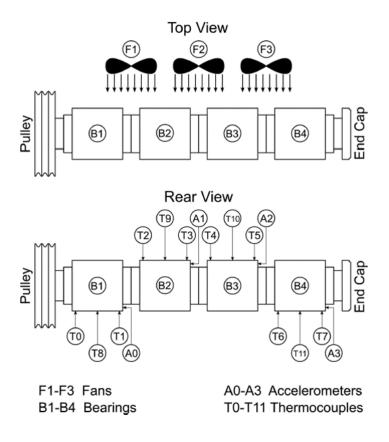
Figure 14: Top and Rear views of 4BT including sensor locations (Montalvo, 2019).
