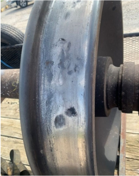
FIGURE 19: WHEEL DEFECTS ON L2 OF AXLE 2
