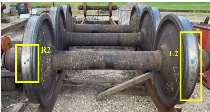
FIGURE 5: AXLE 2 HIGH-CONCERN WHEELSET (DEFECTIVE)
