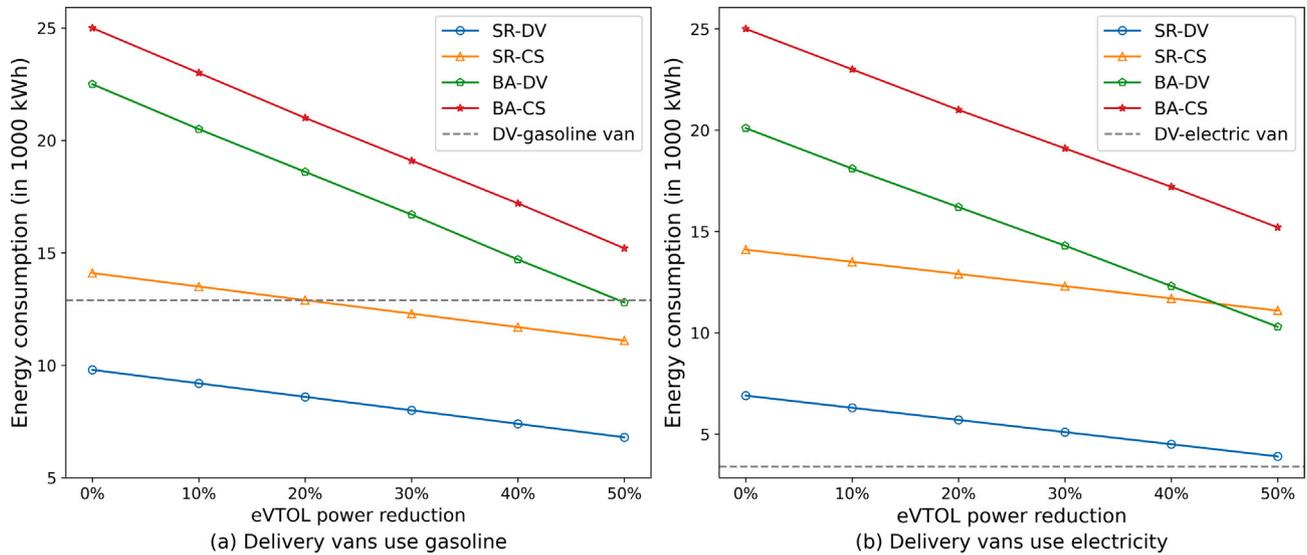
Fig. A.21. Sensitivity of energy consumption to eVTOL power reduction.
