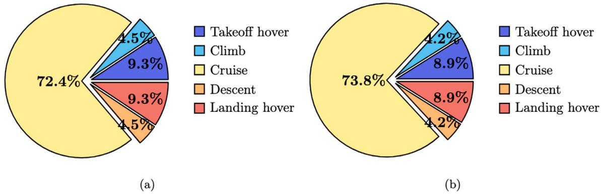
Fig. 13. Energy consumption breakdown for (a) fully-loaded Sabrewing Rhaegal flight profile from the fulfillment center to the vertiport at Woodfield Mall and (b) fully-loaded Beta Alia 250 flight profile from the fulfillment center to the vertiport at Lincolnwood Town Center.
