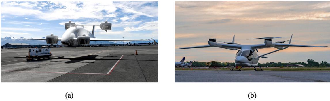
Fig. 1. The two eVTOL types considered in our numerical analysis: (a) Sabrewing Rhaegal B and (b) Beta Alia 250. Source: (Vertical Magazine, 2020; Adams, 2020)
