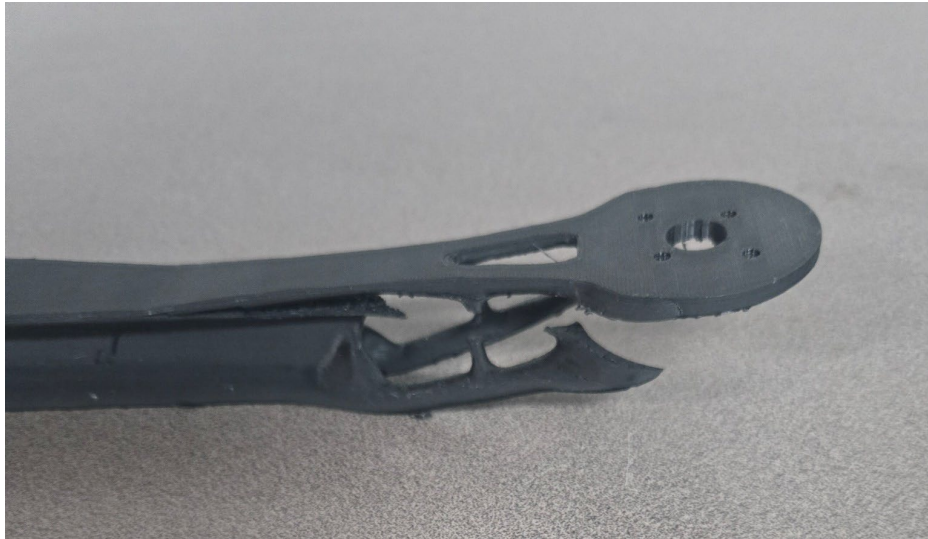
Figure 56: Fractured generatively designed PETG 50% UAV arm following an unintended crash
