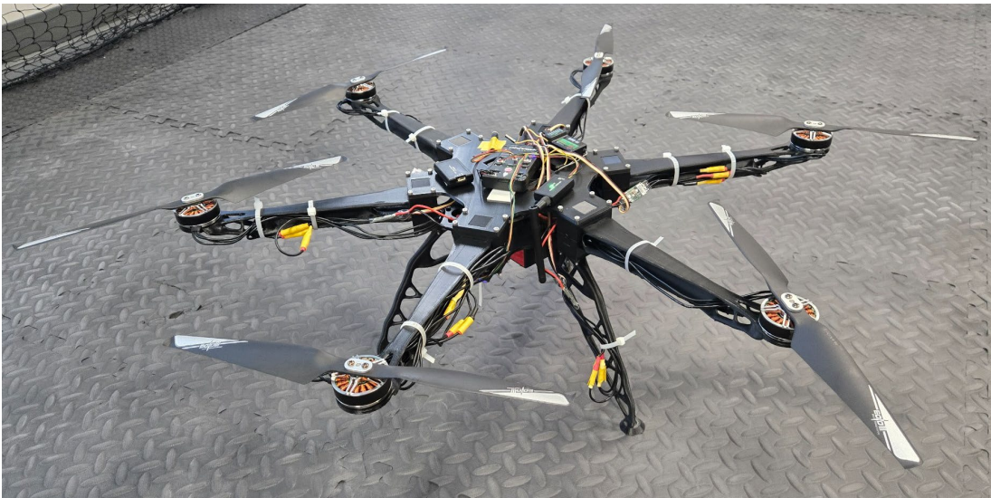
Figure 55: Hexacopter equipped with generatively designed PETG 50% arms during flight
