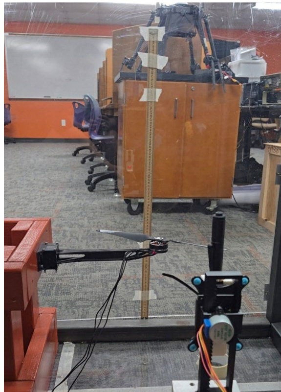
Figure 15: Laser deflection measuring system
