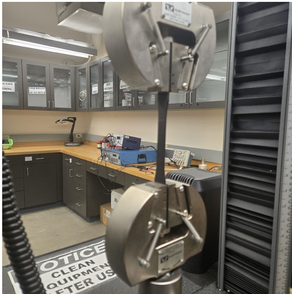
Figure 11: Instron tensile testing setup
