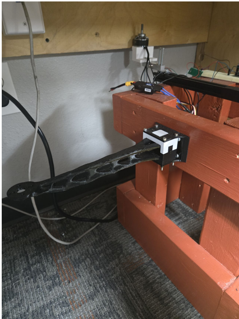
Figure 16: Generated-design specimen on tester
