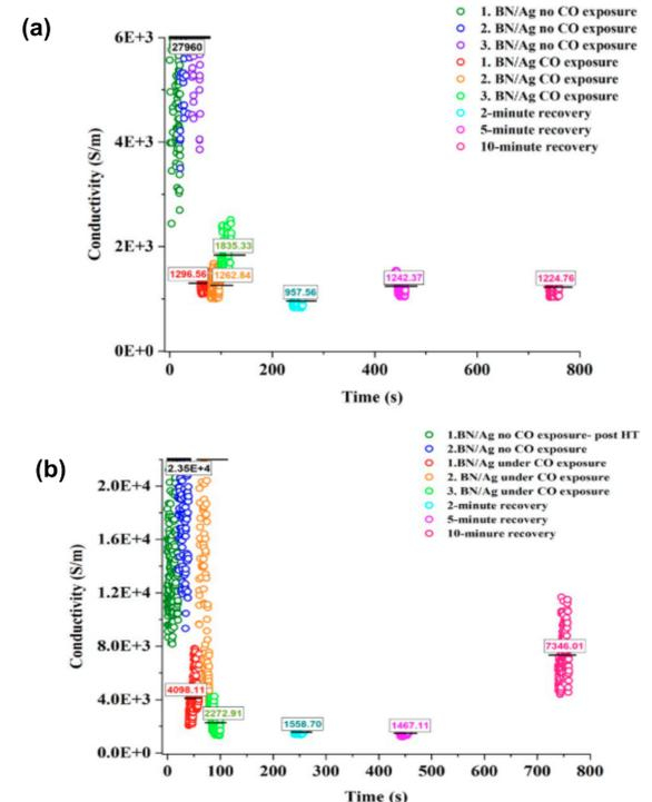
Figure 6- (a) BN/Ag testing with CO gas, (b) BN/Ag testing with CO gas after Hot plate.
