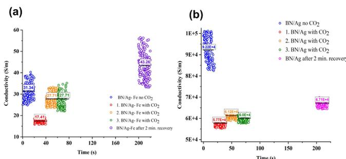
Figure 4 - (a) BN/Ag-Fe and (b) BN/Ag tested with CO<sub>2</sub>
