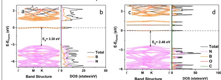
Figure 2 - (a) Electronic band structure for defect h-BN and (b) its densities-of-states (DOS), (c) band structure for defect h-BN with adsorbed CO, and (d) its DOS.
