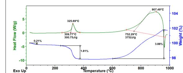
Figure 5 – DSC/TGA analysis for BN- $\text{AgNO}_3$ –PVP system.
