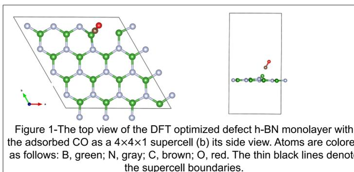
Figure 1-The top view of the DFT optimized defect h-BN monolayer with the adsorbed CO as a  $4 \times 4 \times 1$  supercell (b) its side view. Atoms are colored as follows: B, green; N, gray; C, brown; O, red. The thin black lines denote the supercell boundaries.
