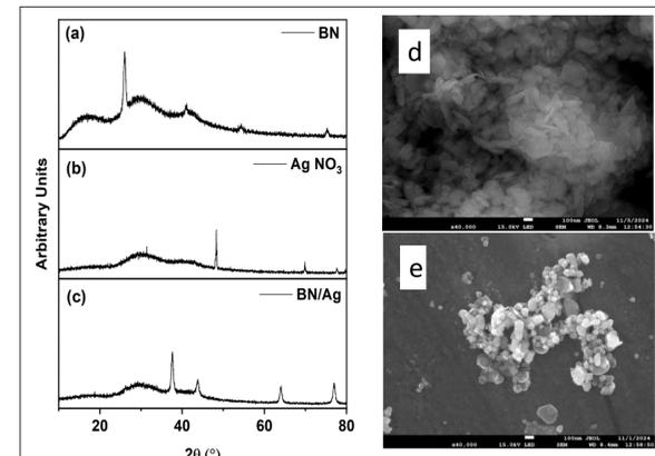
Figure 4- (a,b,c) XRD pattern obtained for nanosized BN,  $\text{AgNO}_3$ , BN- $\text{AgNO}_3$ -PVP, (d) SEM of precursor BN, (e) silver doped BN nanoparticles
