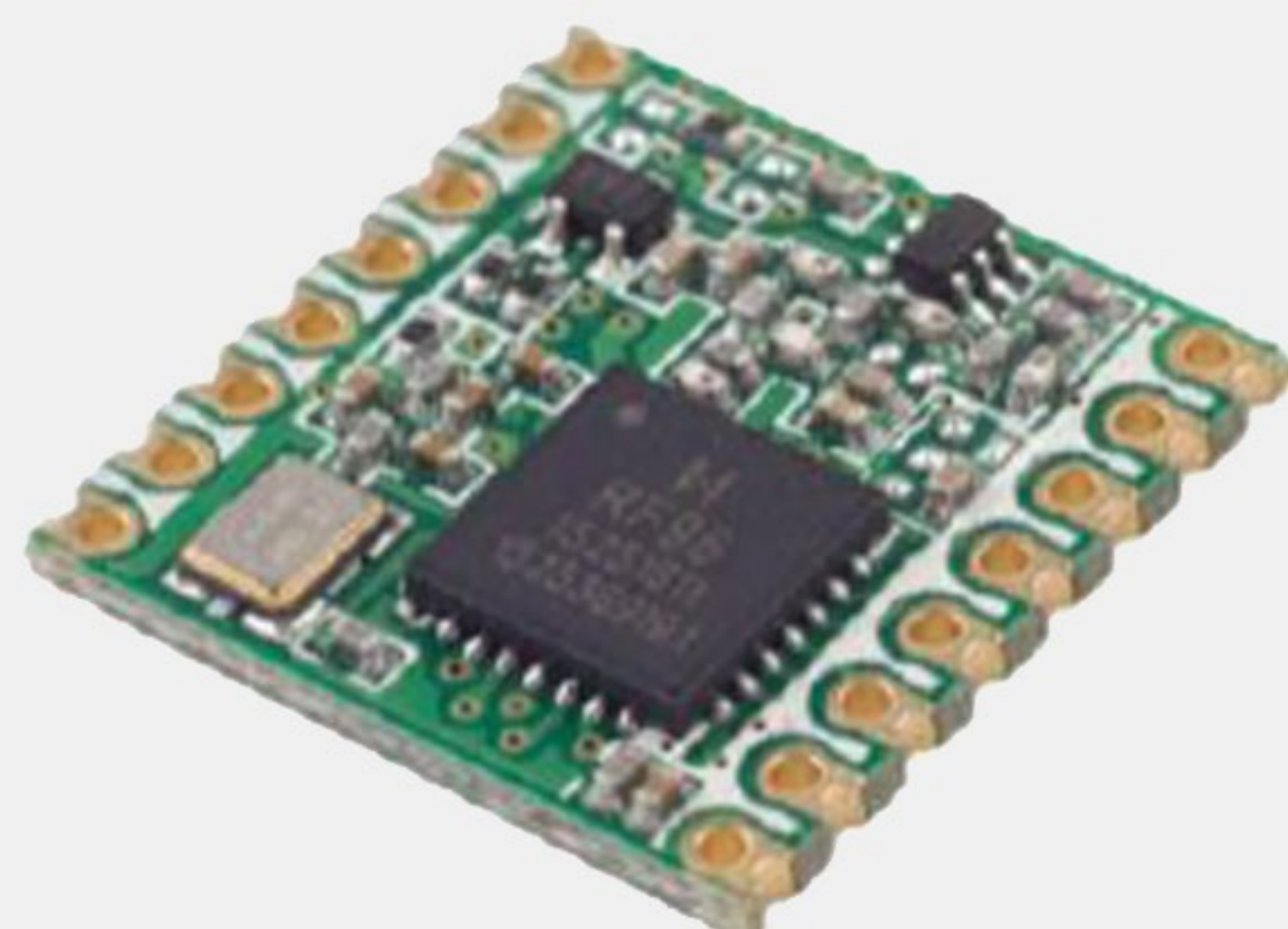
Figure 1. RFM96W LoRa module, 3V Logic Levels, SMD Breakout Board. [1]
