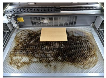
• Using the LC40 screen move the laser head on top of the material.
