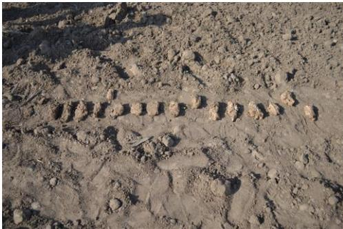
Soil samples from hand-operated auger
