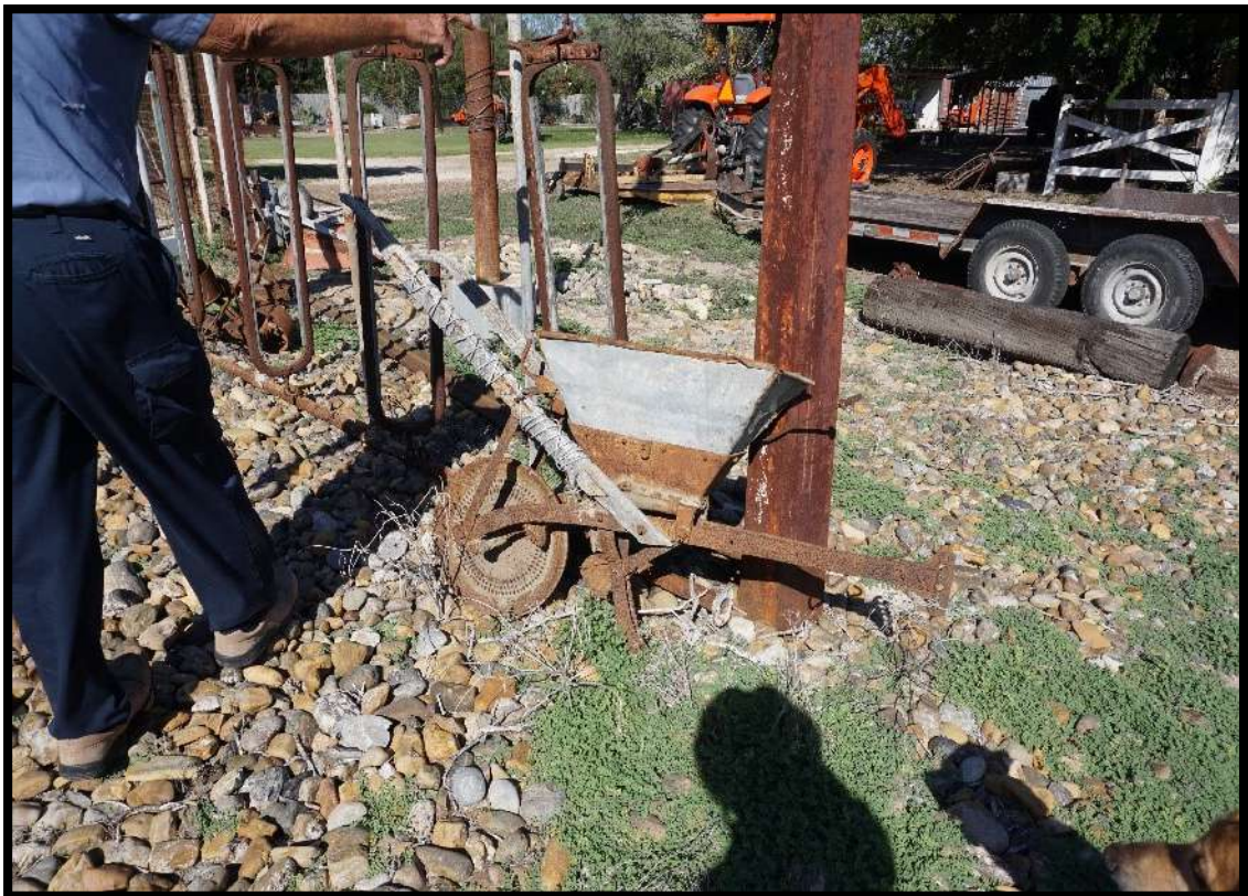
Figure 4.8 Fertilizer machine. Used by Camiel Rogiers. It was pulled by a horse for the vegetable crops, c.1940.
