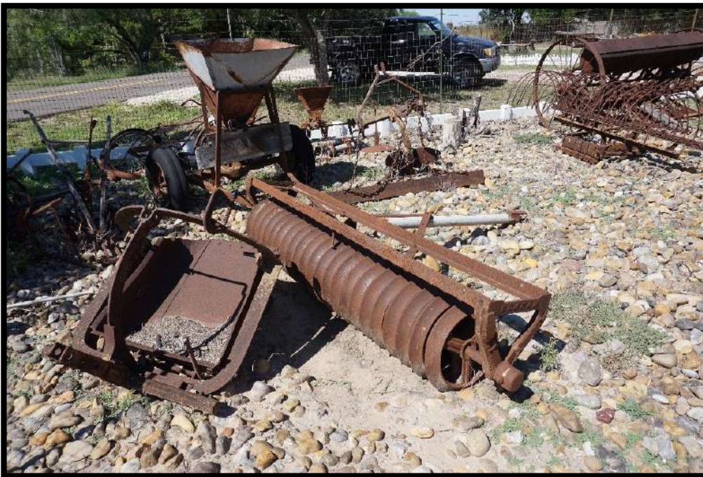
Figure 4.10 "Packer." Equipment used to level the ground after plowing and was pulled by horses. It is no longer in use. Circa 1950's.
