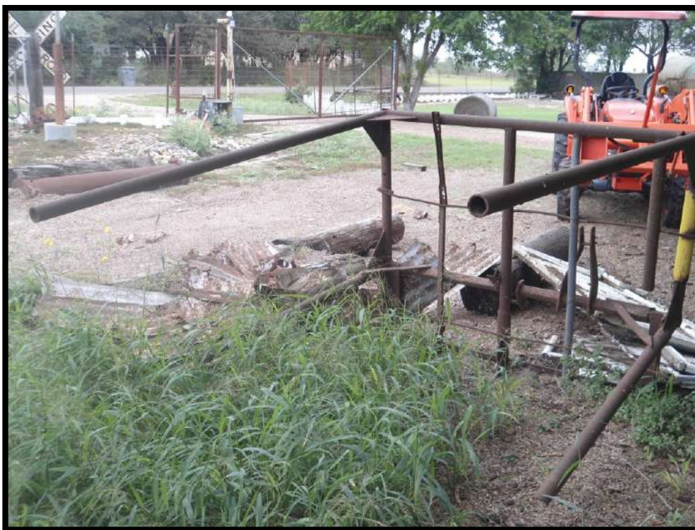
Figure 5.22 Tool that Roy attached to his tractor and use to push brush when clearing land in his orchards. (Courtesy of Jesus Sierra)
