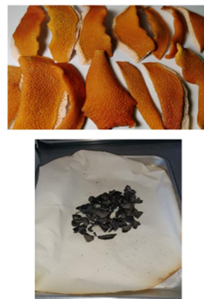
Fig. 2. Grapefruit biomass feedstock and its respective biochar products after pyrolysis at 450°C and 800°C.
