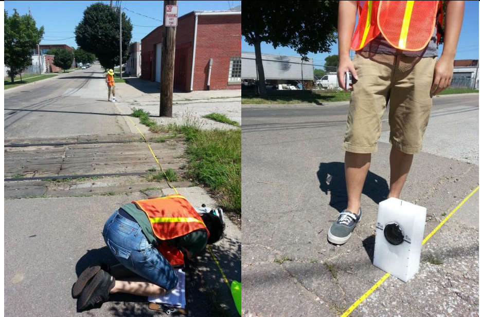
Figure 4.5 Field validation of crossing suitability using a line laser and a retro-reflective lens
