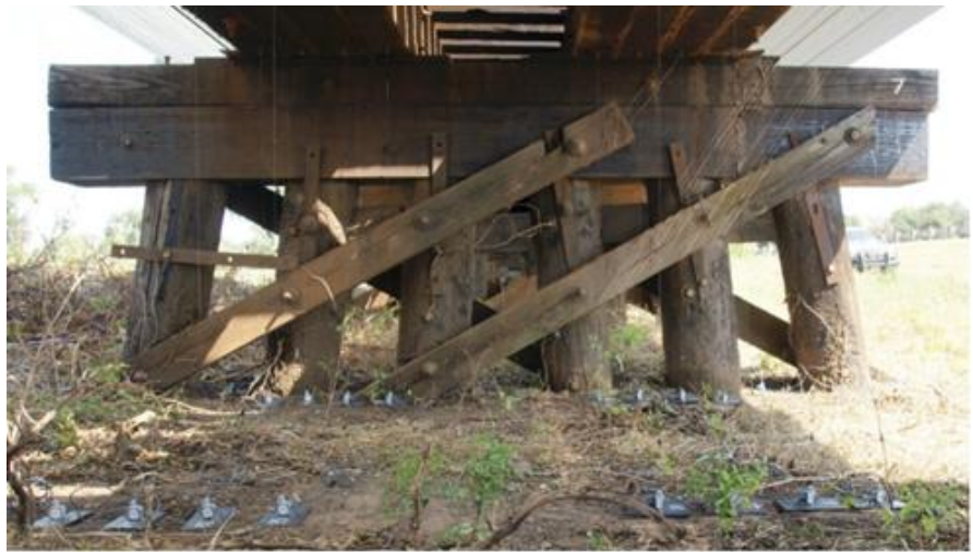
Figure 2: String Potentiometer Setup under Span 7
