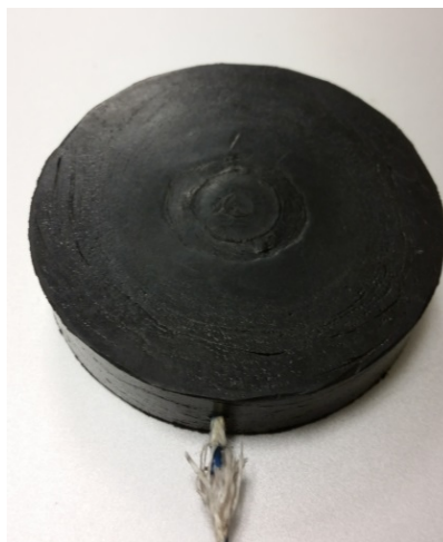
Figure 3: Test Puck of Compounded TPU
