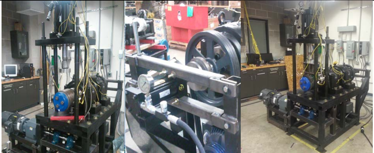
Figure 1: Completed single railroad bearing tester
