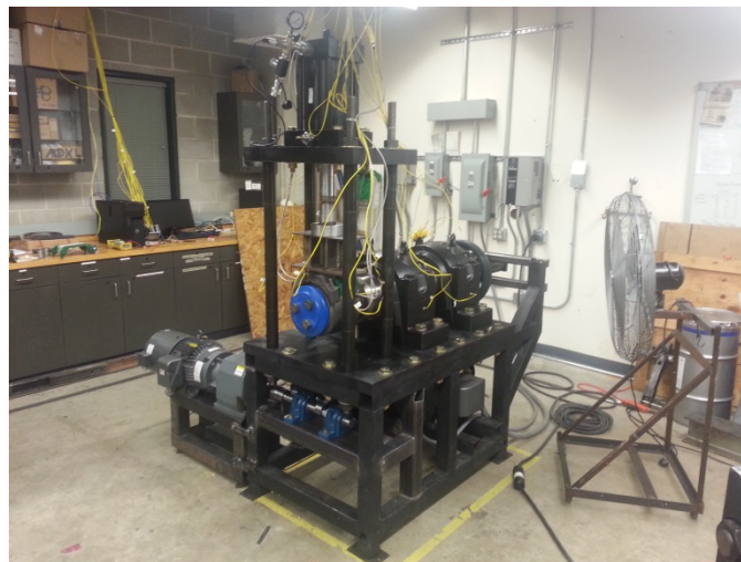
Figure 4: Picture of the Single Bearing Tester with Vertical, Lateral, and Impact Load Capabilities
