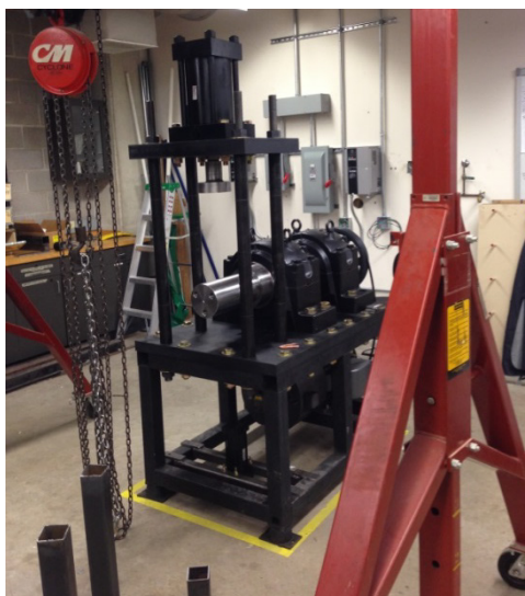
Figure 1. A photograph of the Single Bearing Test Rig with vertical, lateral, and impact loading capabilities.
